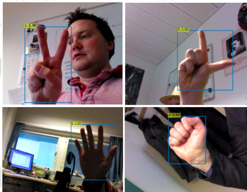
Fig. 4.9: Detection of hand gestures from the OUHANDS dataset in the presence of a human face (top left), background clutter (top right), illumination variation (bottom left), and change in hand orientation (bottom right).
