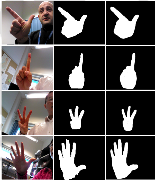
Fig. 2.6: Segmentation results for the Ouhands dataset. The first column contains the input color image, the second contains the ground truth masks, and the third contains the segmented masks.
