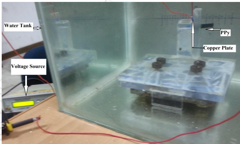
Figure 3.2 Photograph of real time bending experiment under DC voltage
