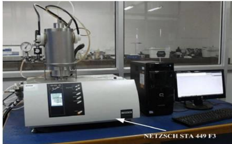
Figure.2.11 Photograph of DSC and TGA Equipment
