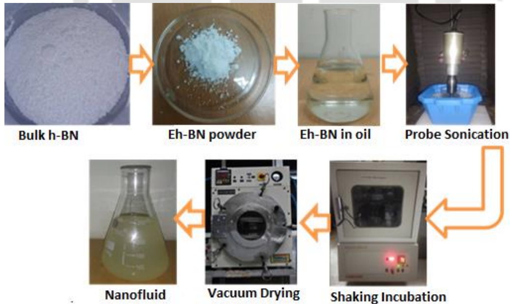
Figure 6.4: Nanofluid preparation with MO/POME.
