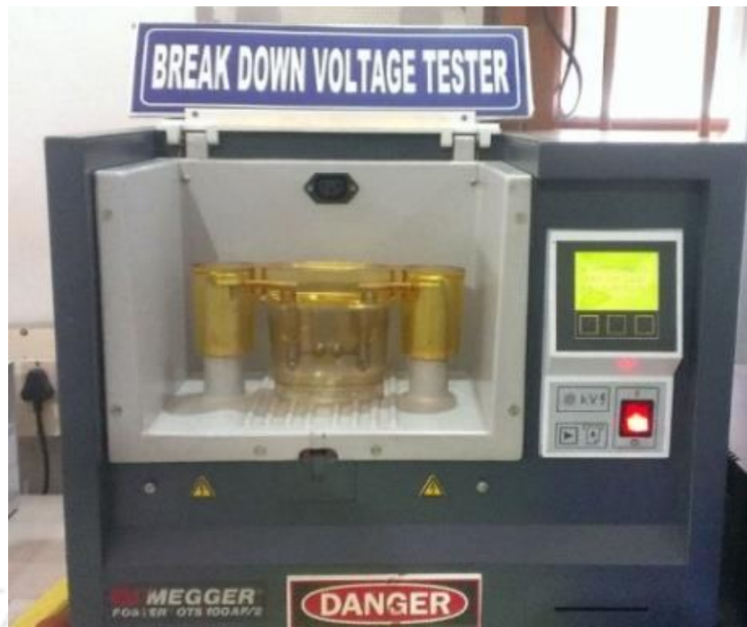
Figure 5.1: ACBDV test setup.
