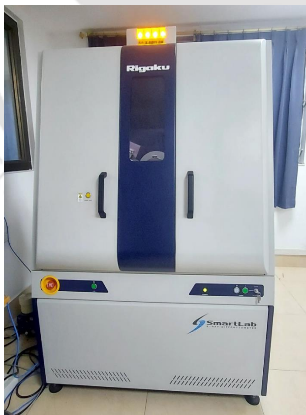
Fig. 2-3 Photograph of the X-ray diffractometer (Rigaku, Smart Lab).
