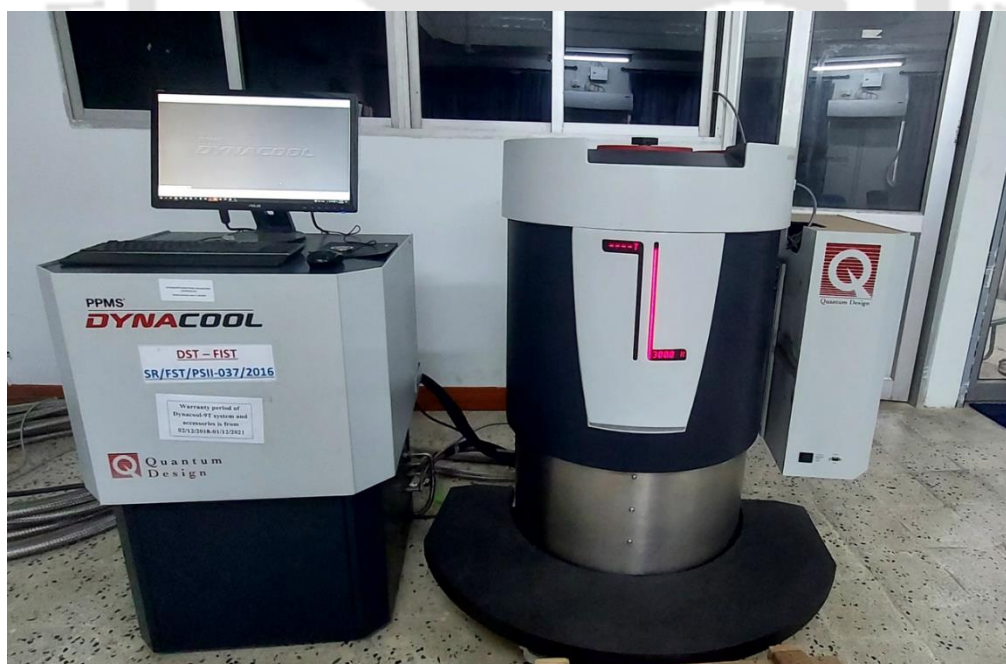
Fig. 2-8 Photograph of physical property measurement system (PPMS, DynaCool).
