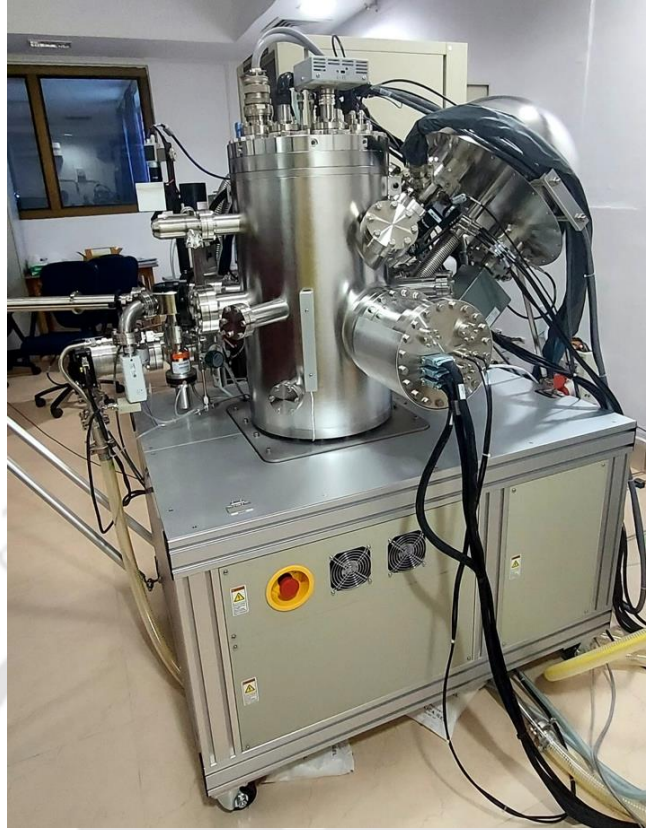
Fig. 2-7 Photograph of the X-ray photoelectron spectrometer (ESCALAB).
