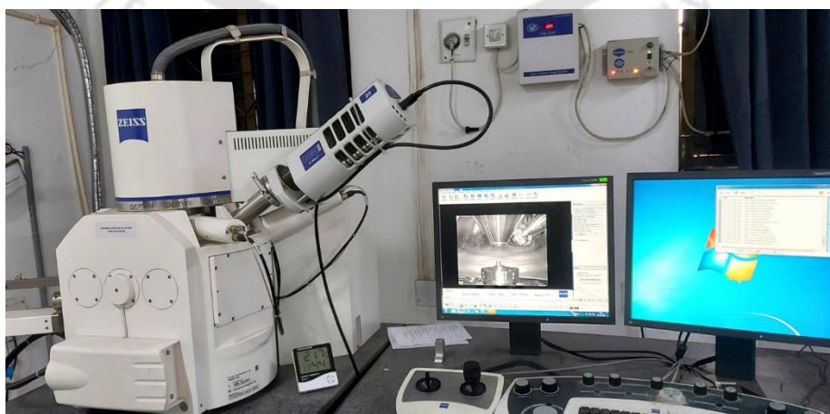
Fig. 2-6 Photograph of the field emission scanning electron microscope (Sigma, Zeiss).
