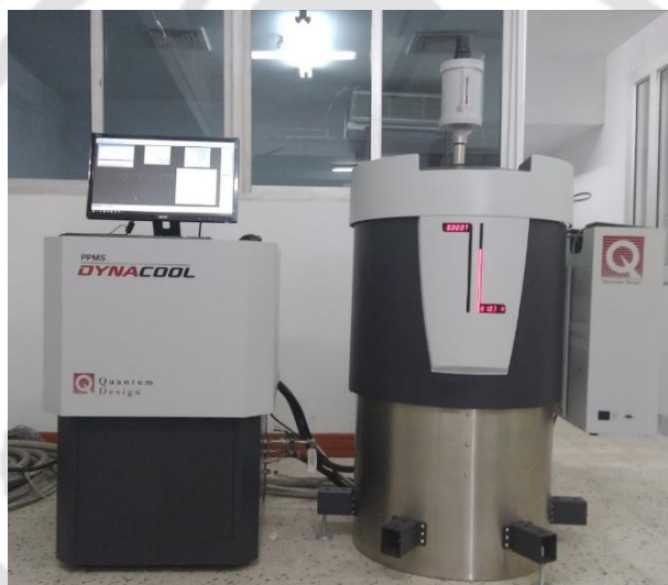
Figure 2.27. Photograph of the 9T PPMS (Quantum Design, Dynacool) with a VSM module.
