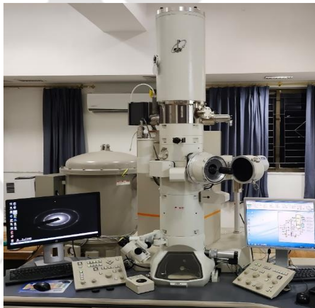
Figure 2.21. Photograph of JEOL-2100F FETEM utilized in this work.
