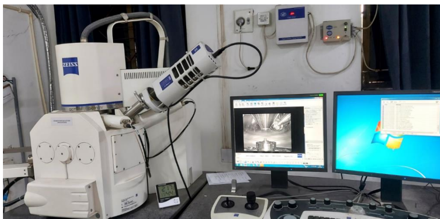
Figure 2.15. Field emission scanning electron microscope (Zeiss Gemini 300).
