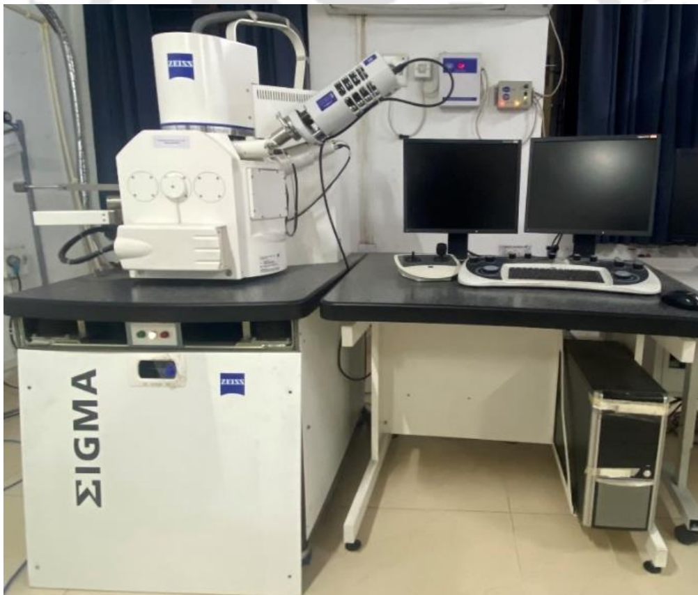
Figure 2.18. Image of an EDS unit attached to Zeiss Sigma FESEM.
