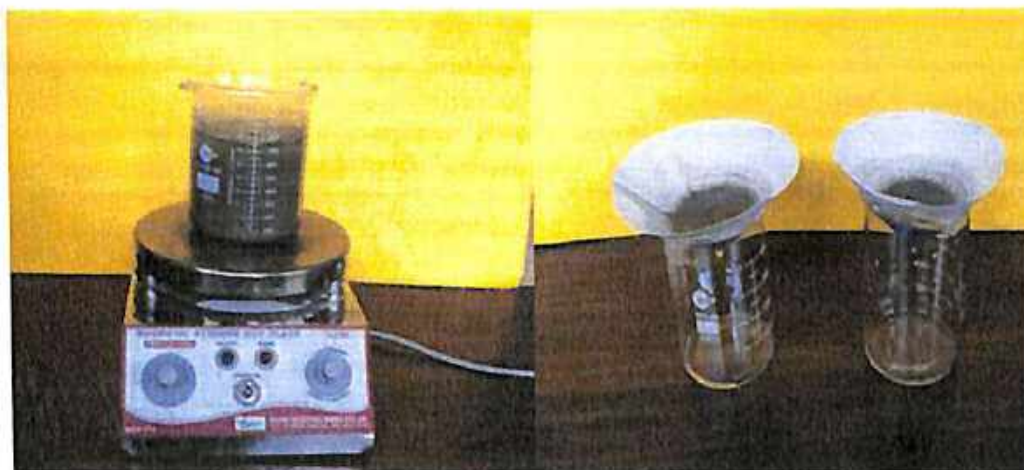
Fig 3.5 Stirring, heating and filtration of electrolytic concrete powder solution extracted from concrete powder
