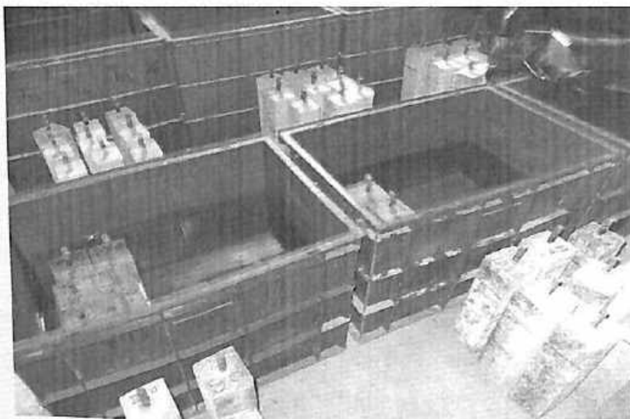
Fig. 3.12 Photograph of reinforced concrete prismatic specimens during wetting and drying
