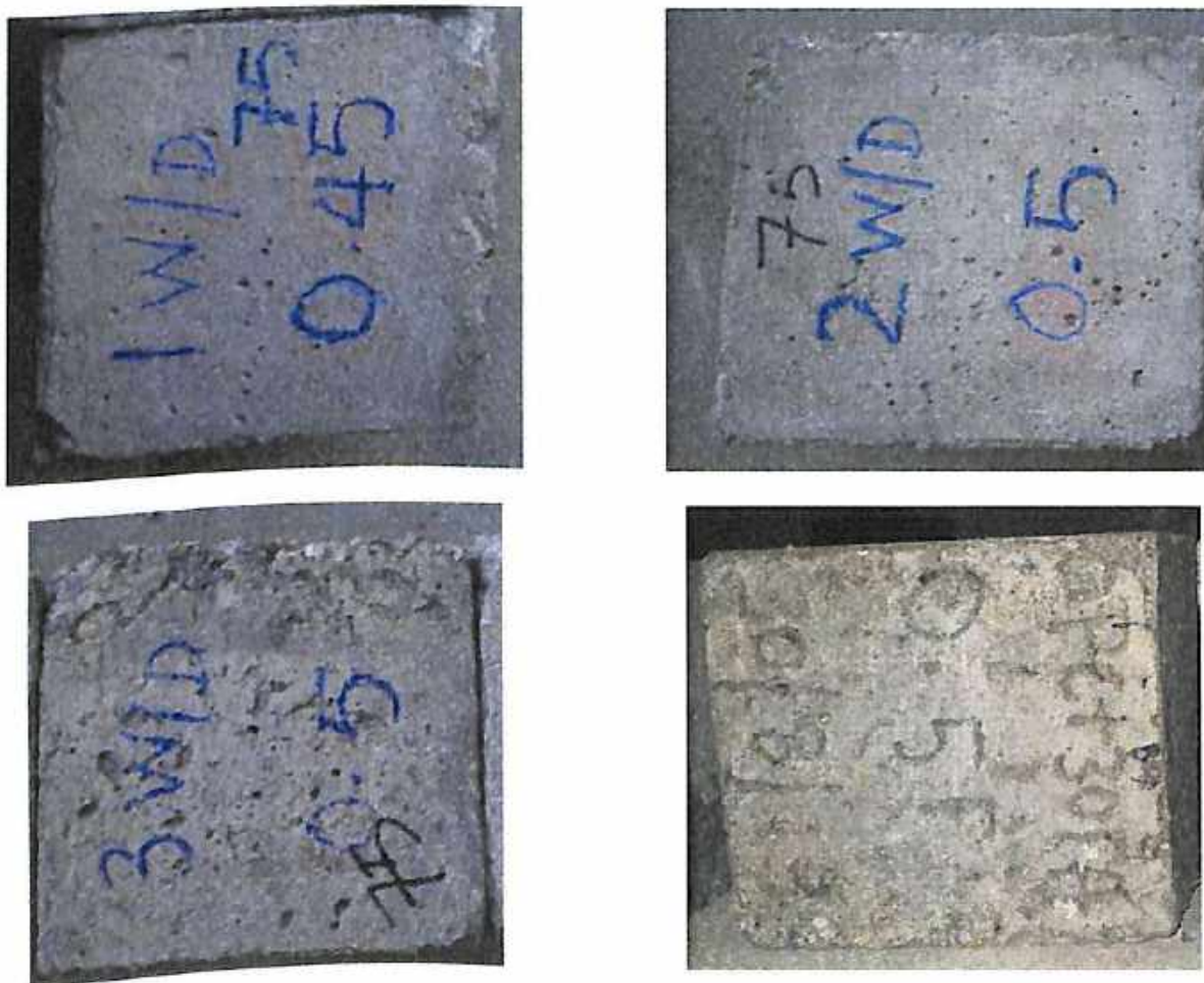
Fig. 7.2 Visual appearance of concrete cube specimens exposed to 12% \text{Na}_2\text{SO}_4 solution with alternate wetting and drying cycles for a period of 360 days
