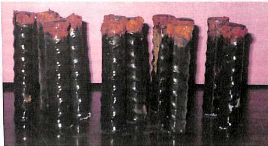
Fig. 3.9 Photograph of steel specimens after completion of potentiodynamic polarization test in contaminated electrolytic concrete powder solution
