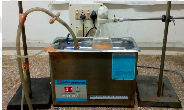
Figure 2.1. Experimental setup for ultrasound-assisted P. rhodozyma fermentation
