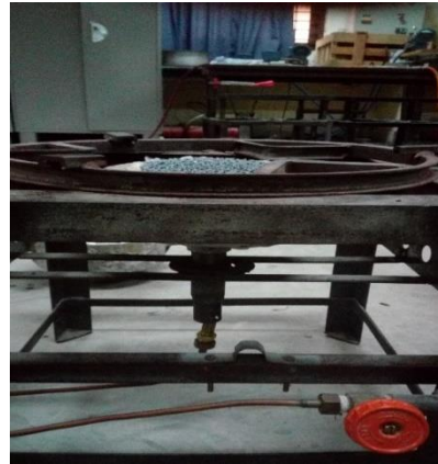
Fig. 4.8: Pictorial view of the cook stove cooking stove with PRB (partially submerged mode).
