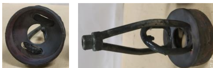
Fig. 6.4: PRB assisted kerosene vaporizer developed by Sinha, 2017.
