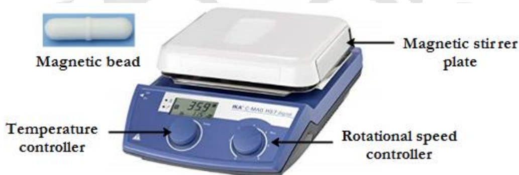
Fig 6.1: Magnetic stirrer (IKAC – Mag, Model: HS7).
