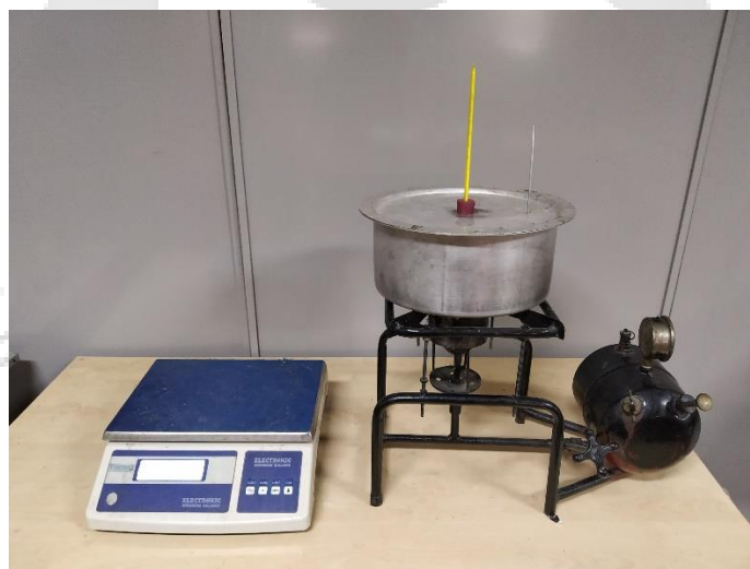
Fig. 6.21: Photographic view of experimental setup for measuring thermal efficiency.
