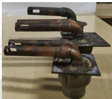
Fig 4.4: Different burner ports (Dia. 15.8 mm, 19 mm and 21 mm ) with connector used in the present work.
