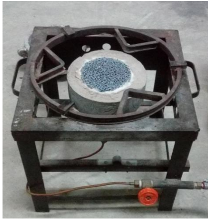
Fig. 4.8: Pictorial view of the cook stove cooking stove with PRB (partially submerged mode).
