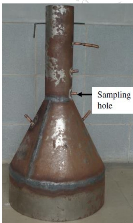
Hood for flue gas sampling
