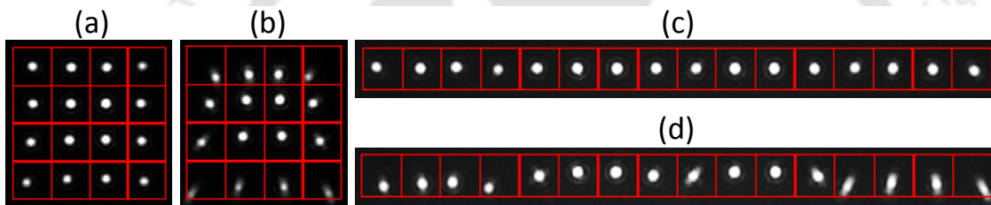
Figure 3.15: The +1 order focal spot array of dimension 4 \times 4 (a) without any holographically added aberration and (b) with holographically added aberration (-1.8 Z_7 ). 1 \times 16 array of +1 order focal spots in the (c) unaberrated case and (d) aberrated case.
