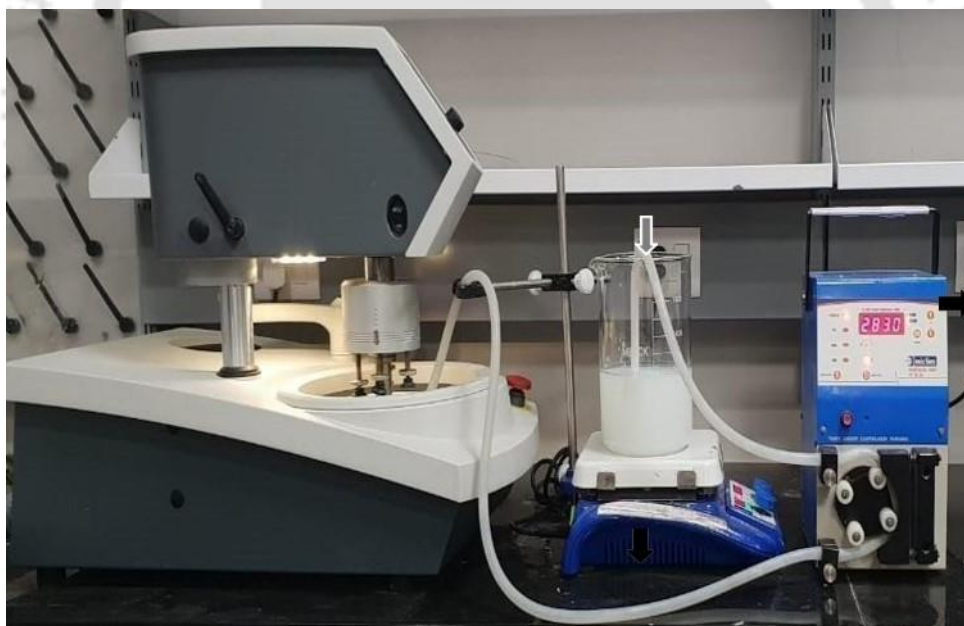
Figure 3.3 Experimental setup including CMP machine for polish rate experiment
