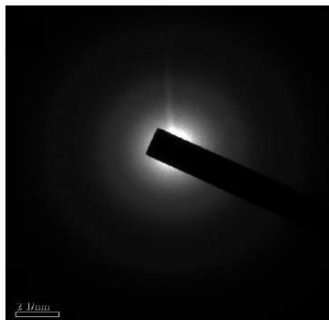
Figure A6.4. Featureless SAED image obtained at 8 min of reaction time after addition of 200 μL, 68.3 mM [Zn 2+ ] to digested Au-NC dispersion.
