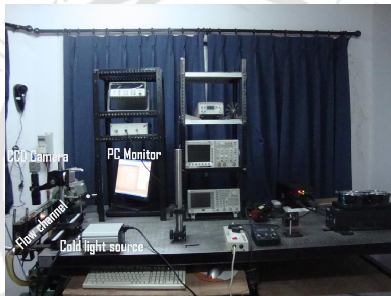
Figure 4.1: Photograph showing the experimental arrangements for capturing images of surface corrugation.
