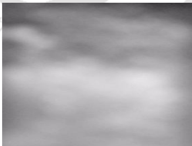
Figure 4.2: A sample image for PSD analysis to characterize the surface corrugation. The sample image was taken for suspension of 250 \mu\text{m} polystyrene particles in the suspending fluid of viscosity 2.05 cP. The volume fraction of the suspension was 0.3.
