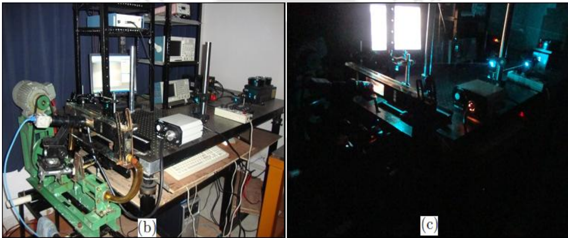
Figure 5.2: (a) Schematic diagram of the experimental setup and optical arrangements for PIV study. (b) (c) Photographs of experimental setup and optical arrangements.
