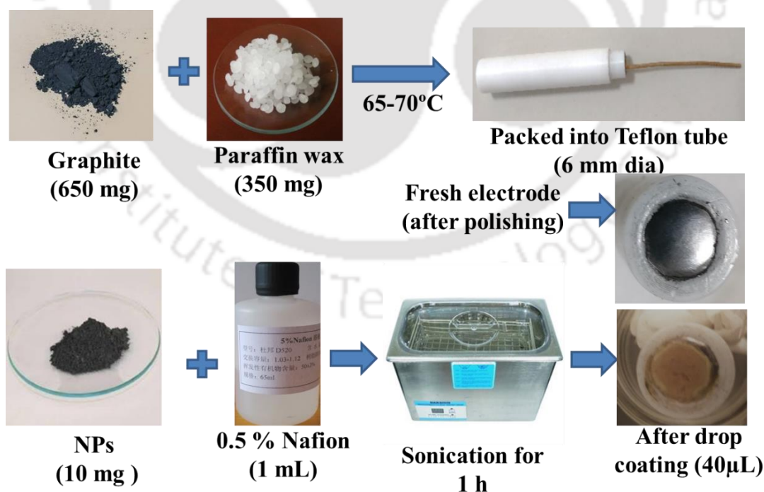
Figure 2.12: Step by step method for the preparation of the working electrode.
