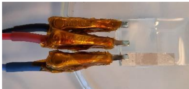
Figure 2.16: Image of the fabricated miniaturized FTO based three-electrode sensing device. The black connector corresponds to the counter electrode, the red connector corresponds to the working electrode and the blue connector refers to the reference electrode (Ag/AgCl).
