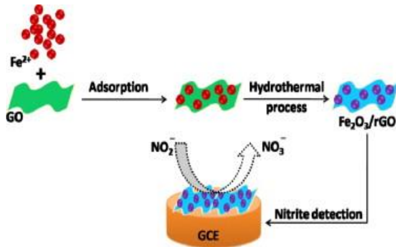
Figure 1.17: Schematic representation of working of electrochemical sensor developed by Radhakrishnan et al. (2014). Reprinted with prior permission. Copyright 2015 Elsevier.
