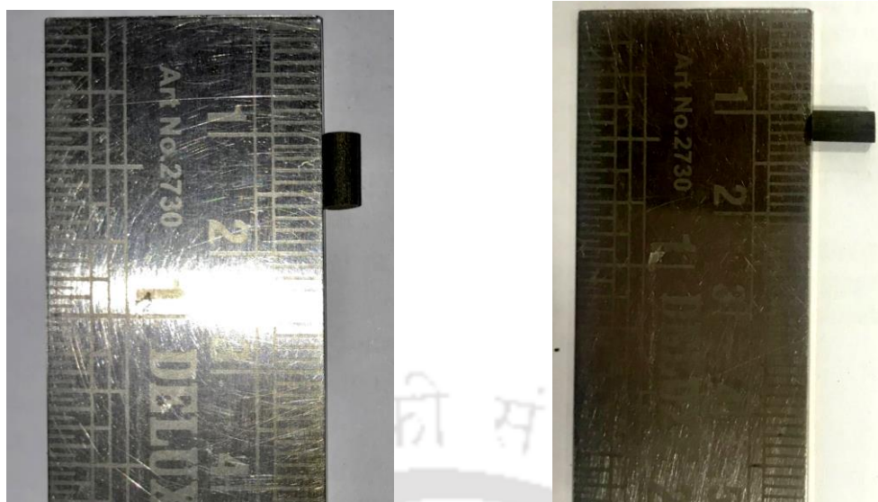
Figure 3. 3. Alloy ingot of WMoVCrTa of \Phi 3 \times 6 mm produced by arc melting
