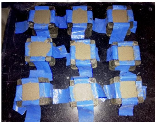
b) Cast cube specimen
