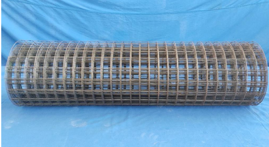
Figure 2.4: Mild steel welded wire mesh
