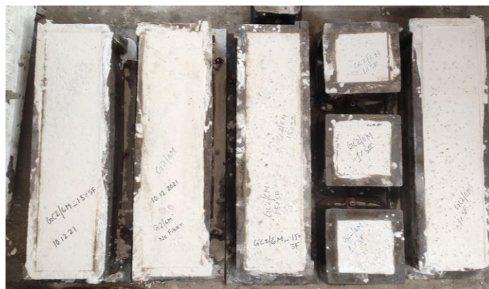
c) Cast cube and prism with FRGC
