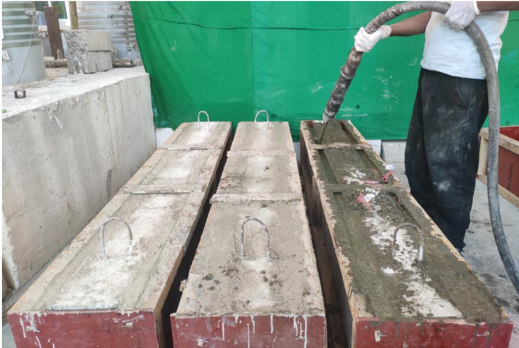
a) Casting process of Jacketed specimen
