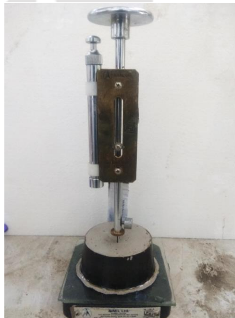
Figure 3.3: Setting time test using Vicat apparatus
