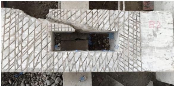
e) Surface preparation around opening
