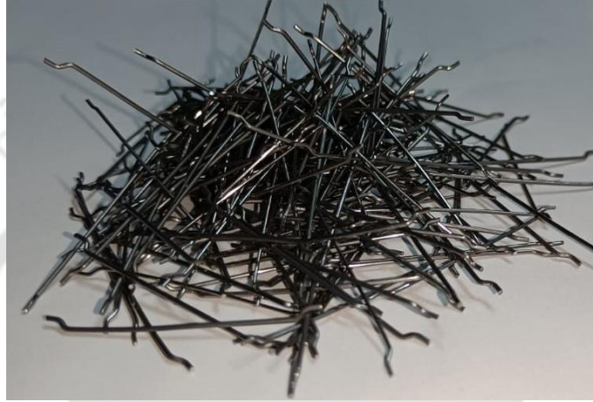
Figure 2.6: Hooked end steel fiber
