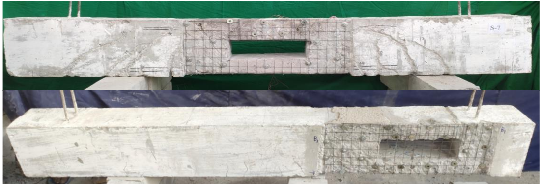
c) Three side wrapping of wire mesh
