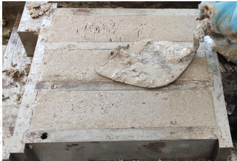
a) Casting of prismatic specimen
