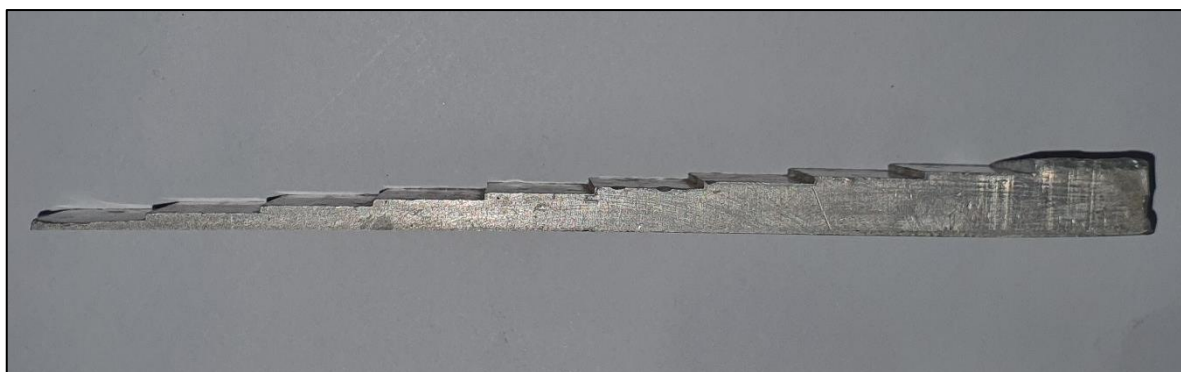
Fig: 3.5. Aluminium 1100 series wedge (1 mm to 10 mm thickness) as a standard reference
