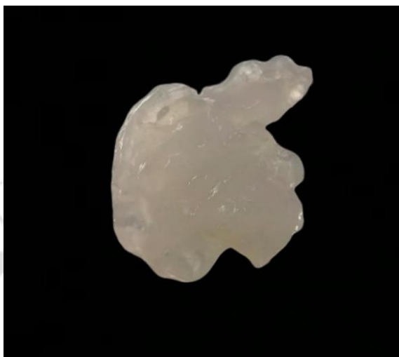
Fig. 5.7 Digital image of the EN-NC-CMC-Na hydrogel obtained via pH-driven addition of EN-NC to CMC-Na solution.
