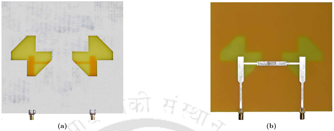
Fig. 4.14: Photograph of the fabricated and tested antenna (a) slotted ground plane (b) feed-lines with IDC
