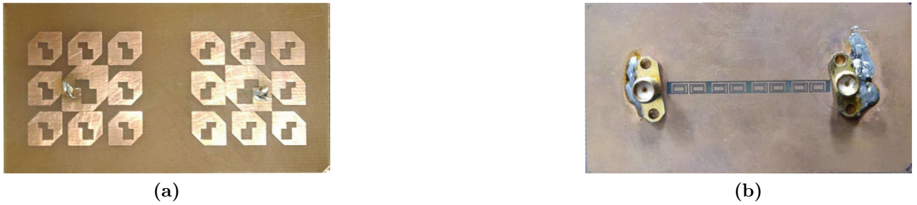
Fig. 6.22: Photograph of the fabricated antenna showing the (a) excited patches surrounded by the parasitic patches and (b) ground plane with the DGS between antenna ports
