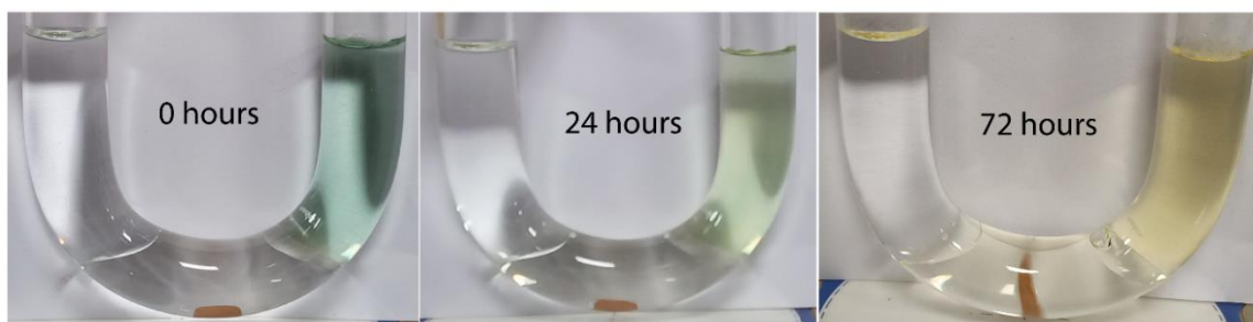
Figure 3.65. Three representative color changes during the U-tube experiment in the presence of the bromothymol blue indicator.
