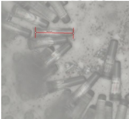
(c) Spin speed: 4000 rpm and UV dosage: 300 mJ/s
