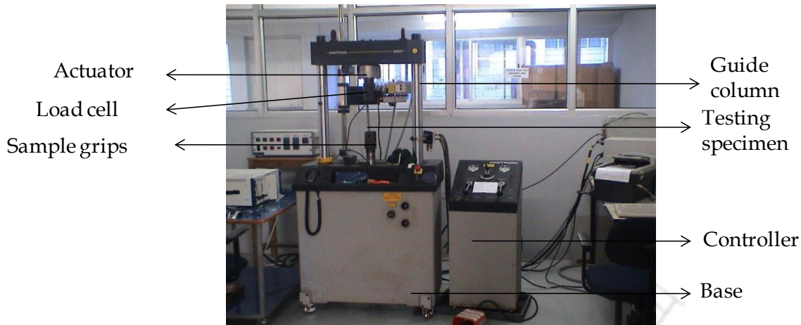
Fig. 3.12 INSTRON universal testing machine with closed loop servo hydraulic system.
