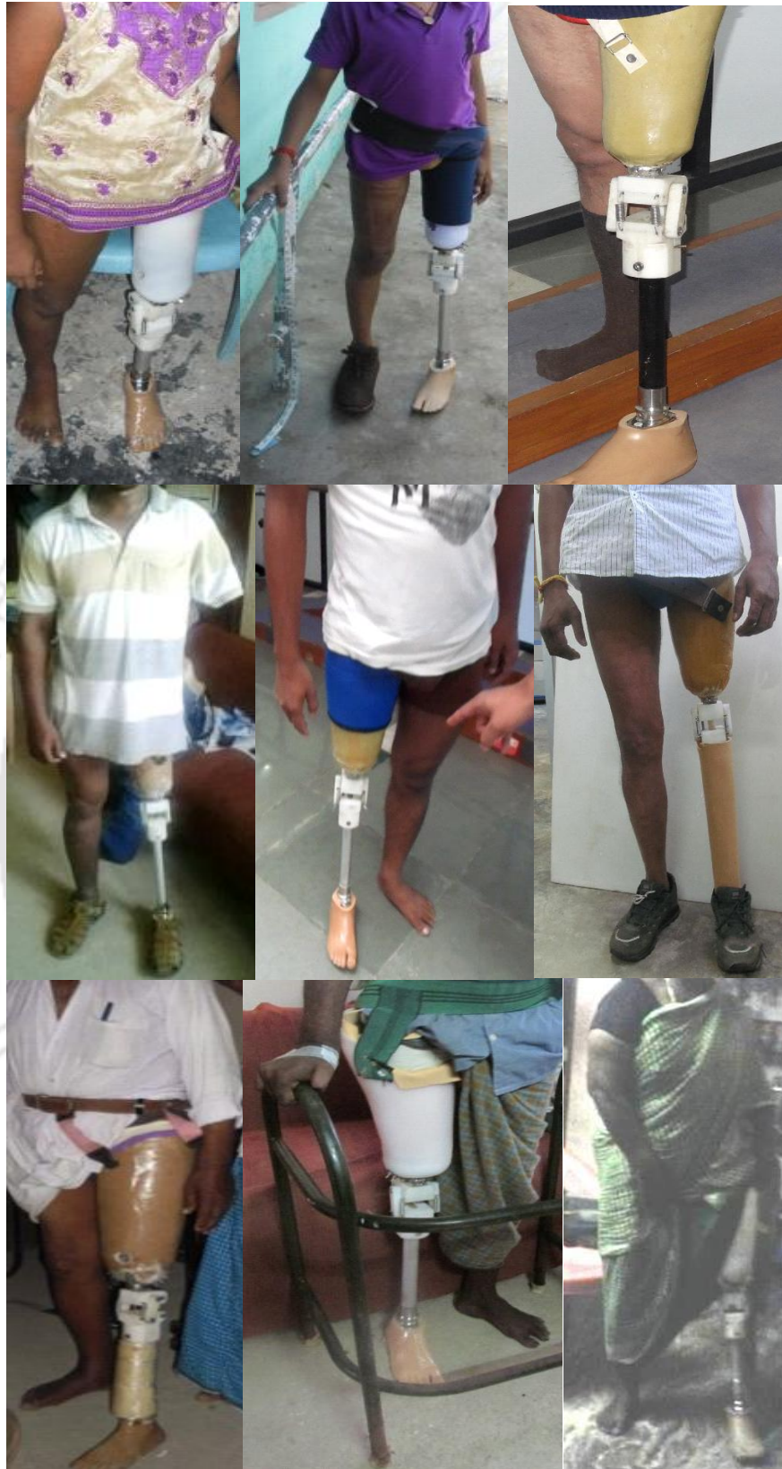
Fig. 4.20 Photographic view of all nine amputees fitted with the developed prosthetic knee joint
