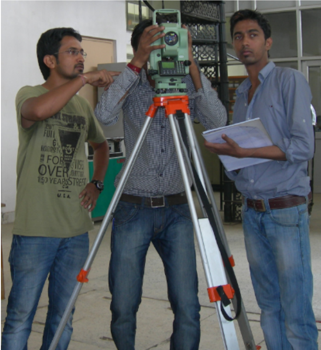
FIGURE 2.9: Measurement of bed slope by total station
