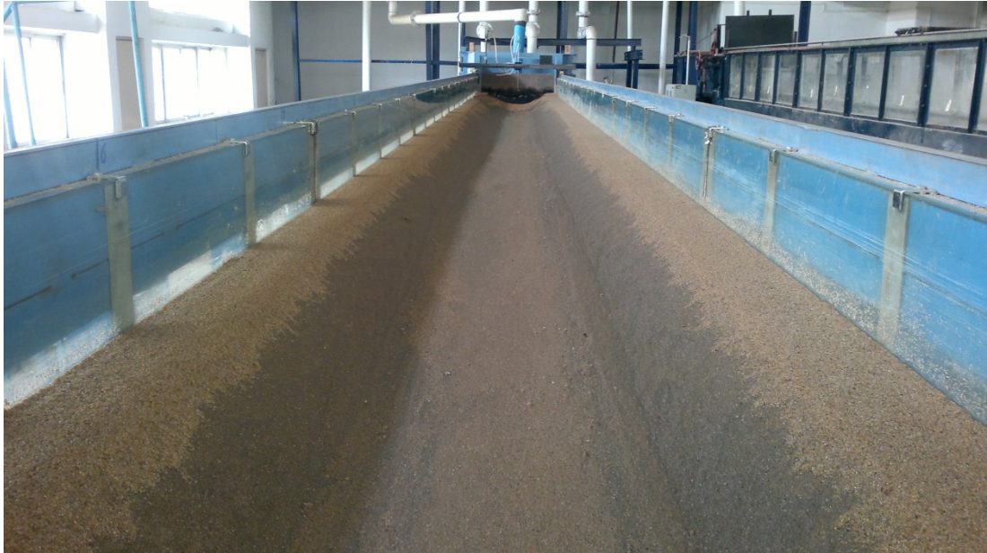
FIGURE 2.21: Channel after seepage experiment on the sand of d_{50} = 0.62 mm
