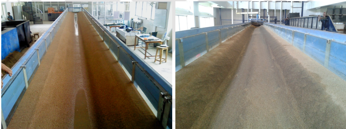
FIGURE 3.15: Snapshot of the channel after (A) no seepage experiment and (B) seepage experiment
