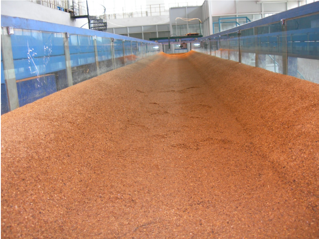
FIGURE 2.20: Channel after seepage experiment on the sand of d_{50} = 1.1 mm
