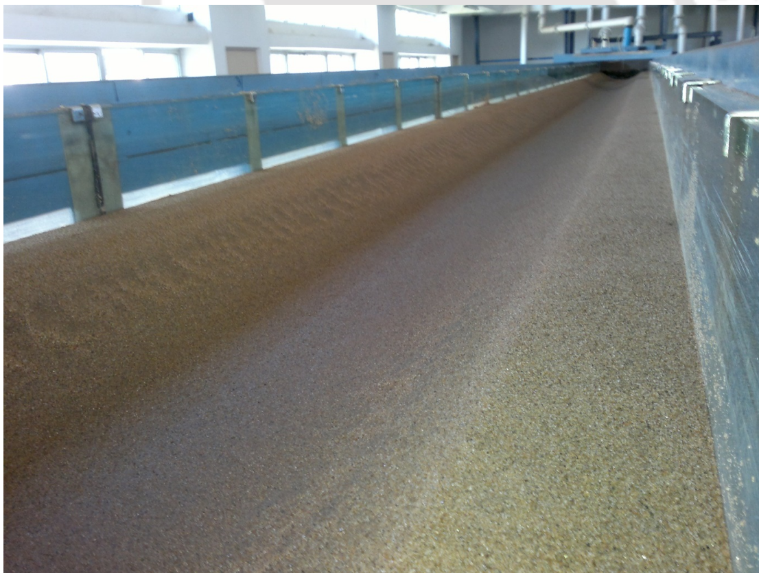
FIGURE 3.38: Undistorted channel bank obtained after the no seepage experiment
