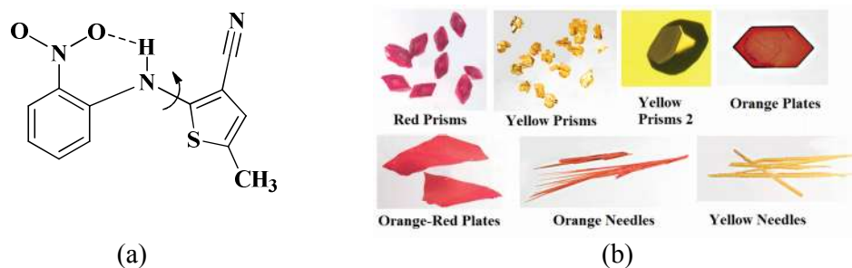
Figure 2.1: (a) Structure of 5-methyl-2-[(2-nitrophenyl)amino]-3-thiophenecarbonitrile (ROY) (b) Polymorphs of ROY showing different colors and shape.
