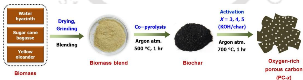
Figure 5.1 Synthesis protocol of oxygen-rich porous carbon (PC- x ) from blends of sugarcane bagasse, water hyacinth, and yellow oleander.
