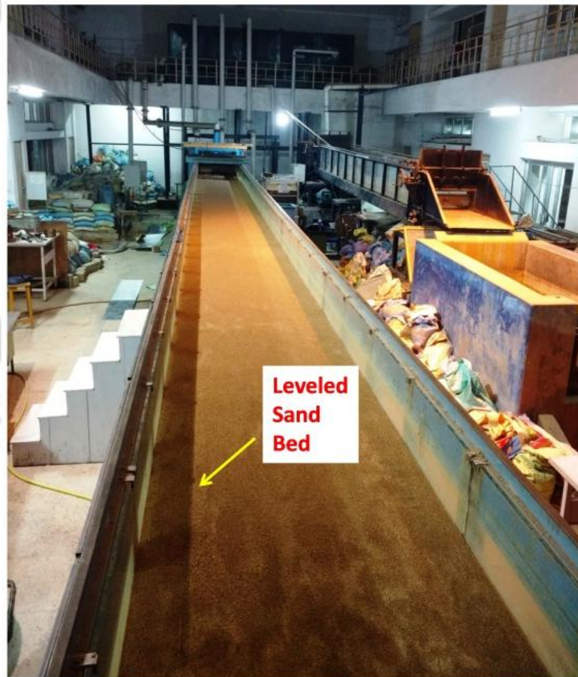
Figure 2.9 Preparation of sand bed with metal cutter
