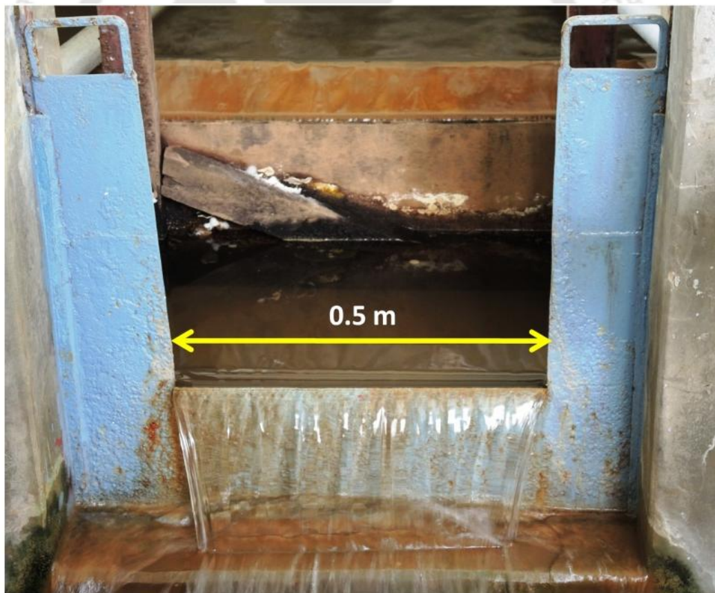
Figure 2.3 Rectangular notch for discharge measurement
