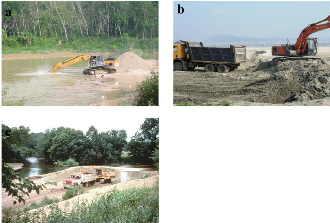
Figure 1.2 (a) Wet-pit mining in Sungai Kulim, Penang, Malaysia (Langer, 2003) (b) Dry-pit mining in Bhramaputra River near Saraighat bridge, Guwahati, Assam, India (photographed by the author, 2018) (c) Bar-skimming in Sungai Kulim, Penang, Malaysia (Langer, 2003).
