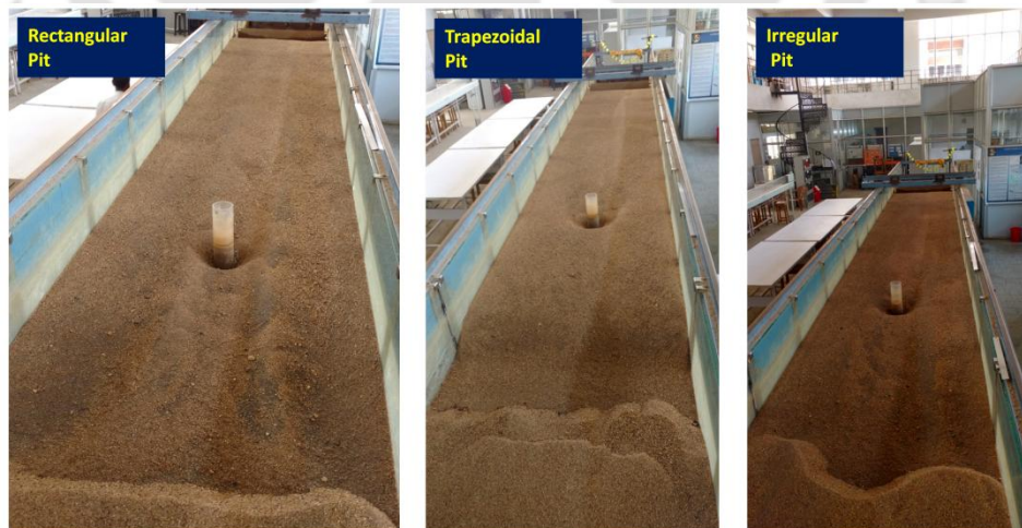
Figure 2.12 Snapshots of pit migration and morphology around pier for all three pit shapes at Q = 0.0567 \text{ m}^3/\text{s} .
