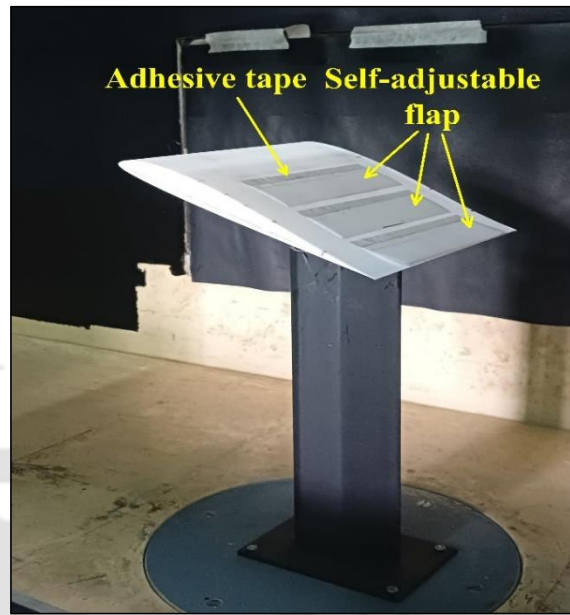
(b) Multiple flaps configuration
