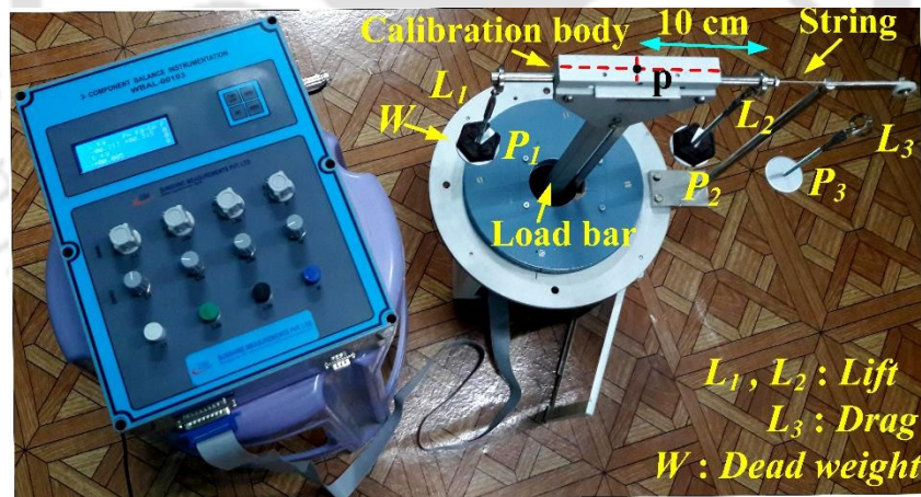
Fig. 3.4: Calibration setup for force balance
