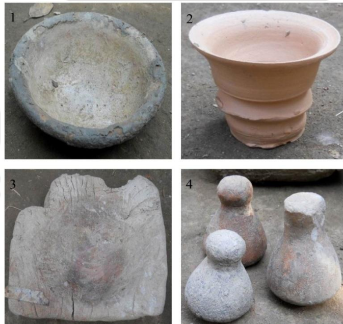
Figure 4.4 Various tools: 1) Earthen bowl (Aphori, use for shaping xaneki/saru and the base of other pots) 2) Clay item (it is known as "majani", use to make the outer surface of the pots more smooth.) 3) Wooden Plate (Local term is "Aathali", use for shaping the earthen wares) 4) Tools made of cement or stone, it is use to give shape to the pots and also use to make the surfaces smooth. In local term it is known as "Bolia".
