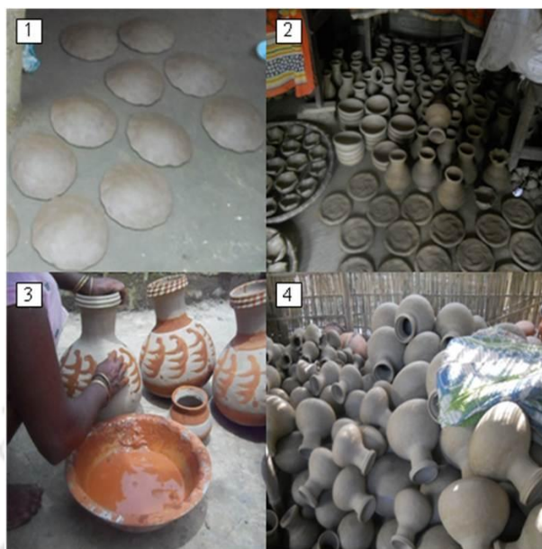
Figure 4.8 Hira potters' Manufacturing process 1. Base 2. Some finish products and bases 3. Coloring pots with Geru before firing 4. Unfired finished products stored in shed
