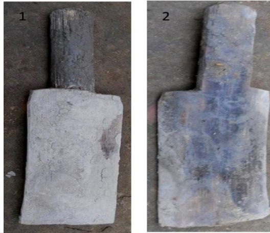
Figure 4.7 Wooden beater: front and Back view (it is locally known as Pitani, use to give shape to the wares)
