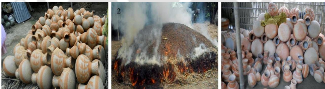
Figure 4.9 Hira Pottery: 1) Piled for firing 2) Firing process 3) After firing
