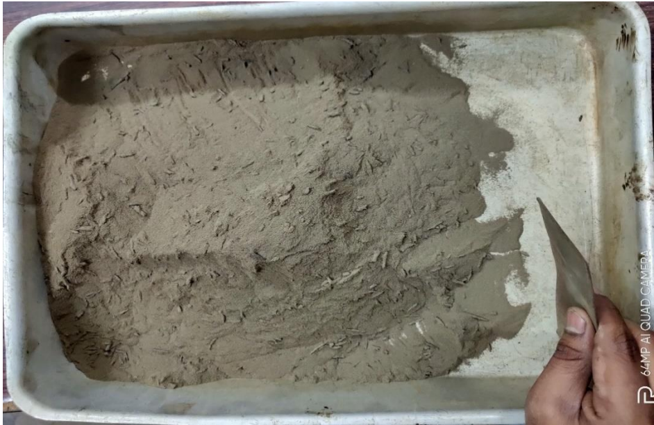
Fig. 3.9. BC soil-tire fibre mix.
