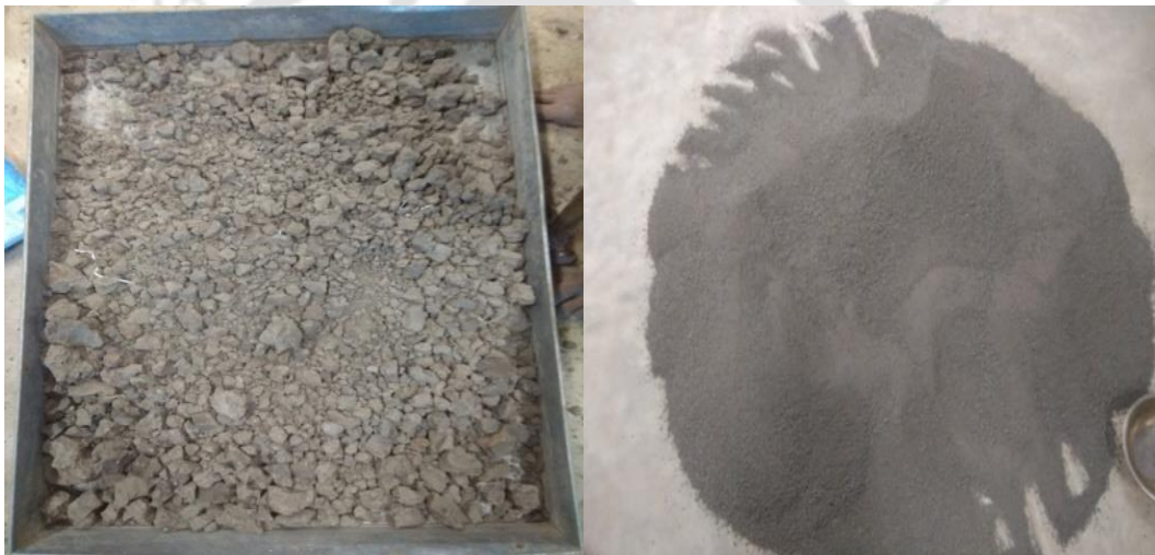
Fig. 2.4. Black cotton soil (before and after pulverization).
