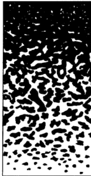
Fig. 1.1 Schematic diagram of functionally graded material (FGM) (Markworth et al. 1995).
