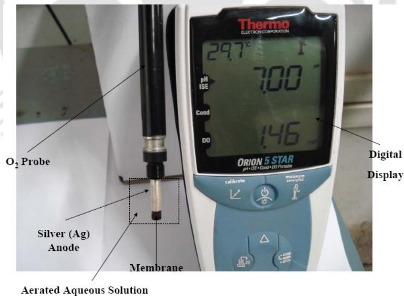
Figure 2.6: Oxygen molecules pass through the semi permeable silicon membrane into the electrolyte solution surrounding the electrodes
