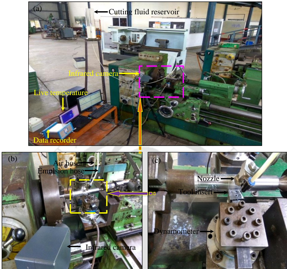
Figure 6.3. (a) Overview of MQCF experiment setup, (b) magnified view of the infrared camera, emulsion-air hoses, tooling, etc. and (c) magnified view of the tool-workpiece-mist interaction
