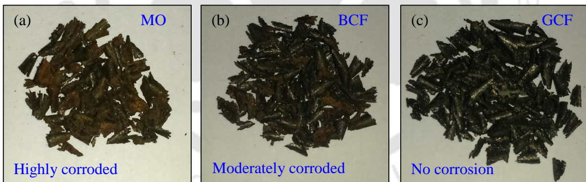
Figure 5.13. Tested chips with 2.5 % concentration of (a) mineral oil, (b) bio-cutting fluid and (c) green cutting fluid
