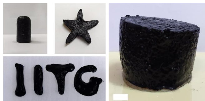
Figure 4.2. Template assisted gel casting of MGH hybrid for desired shape. The scale bar is 1 cm.
