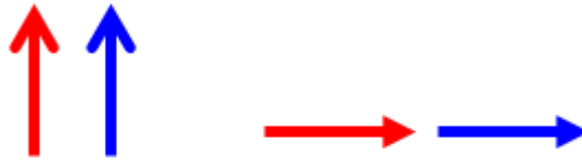
Figure 2.08: Schematic drawing of broadside and head-to-tail configurations for a pair of ferromagnetically coupled magnetic moments [PERU20131].
