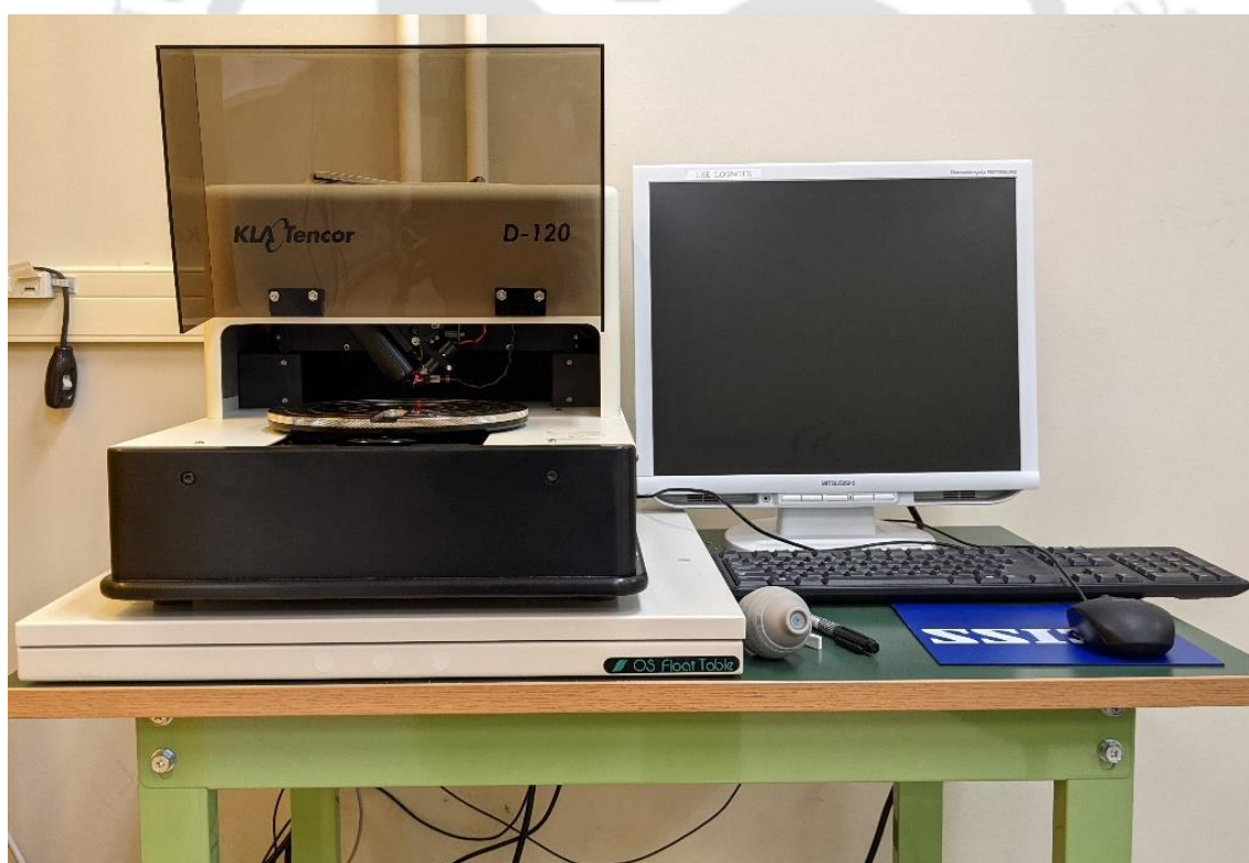
Figure 3.06: Photographic view of KLA-Tencor D-120 stylus profilometer used in the present investigation [NIMS2019].
