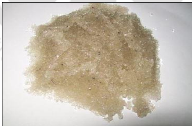
Figure 6.2: Sample of glass beads used in the study
