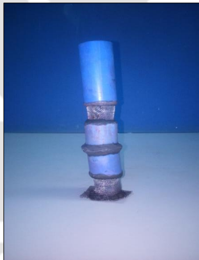
Figure 6.4: Groundwater circulation well (GCW) used in the present study
