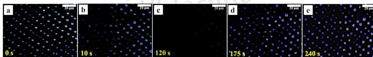
Figure 5.7 Polarized optical microscope image of 5CB filled array of microwells, serve as light-reflecting pixels. Upon exposure to the solvent (n-hexane), the nematic to isotropic (N-I) transition takes place at 120 s (Figure
