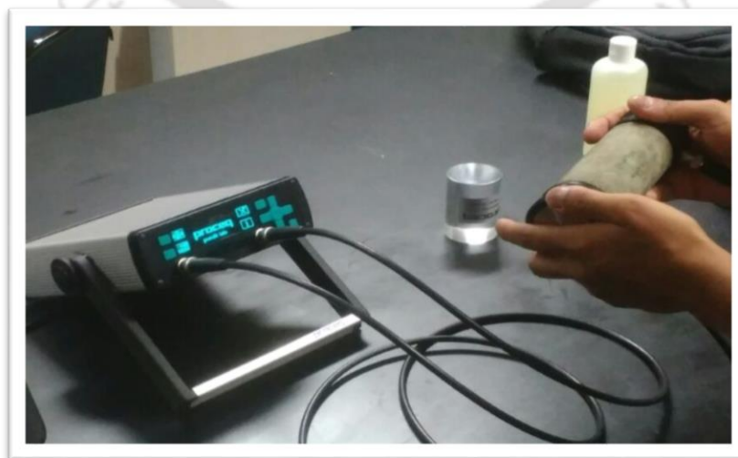
Figure 3.2 Determination of V_p in laboratory for rock core plugs by PUNDIT setup
