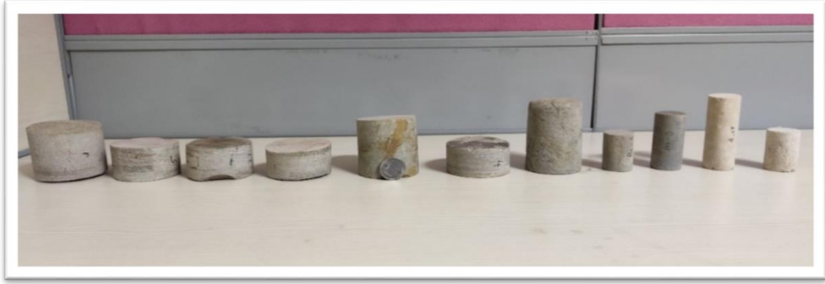
Figure 3.3 Core samples collected for performing ultrasonic pulse velocity measurement (A1 to A11 from left to right)
