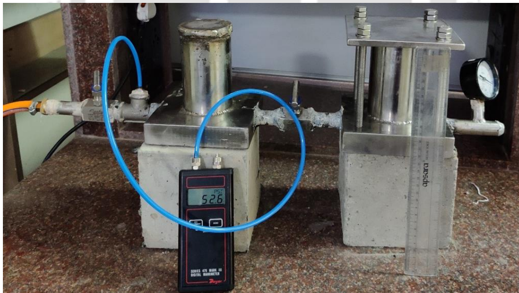
Figure 3.9 Helium Gas Porosimeter (HGP) setup as elaborated in this study
