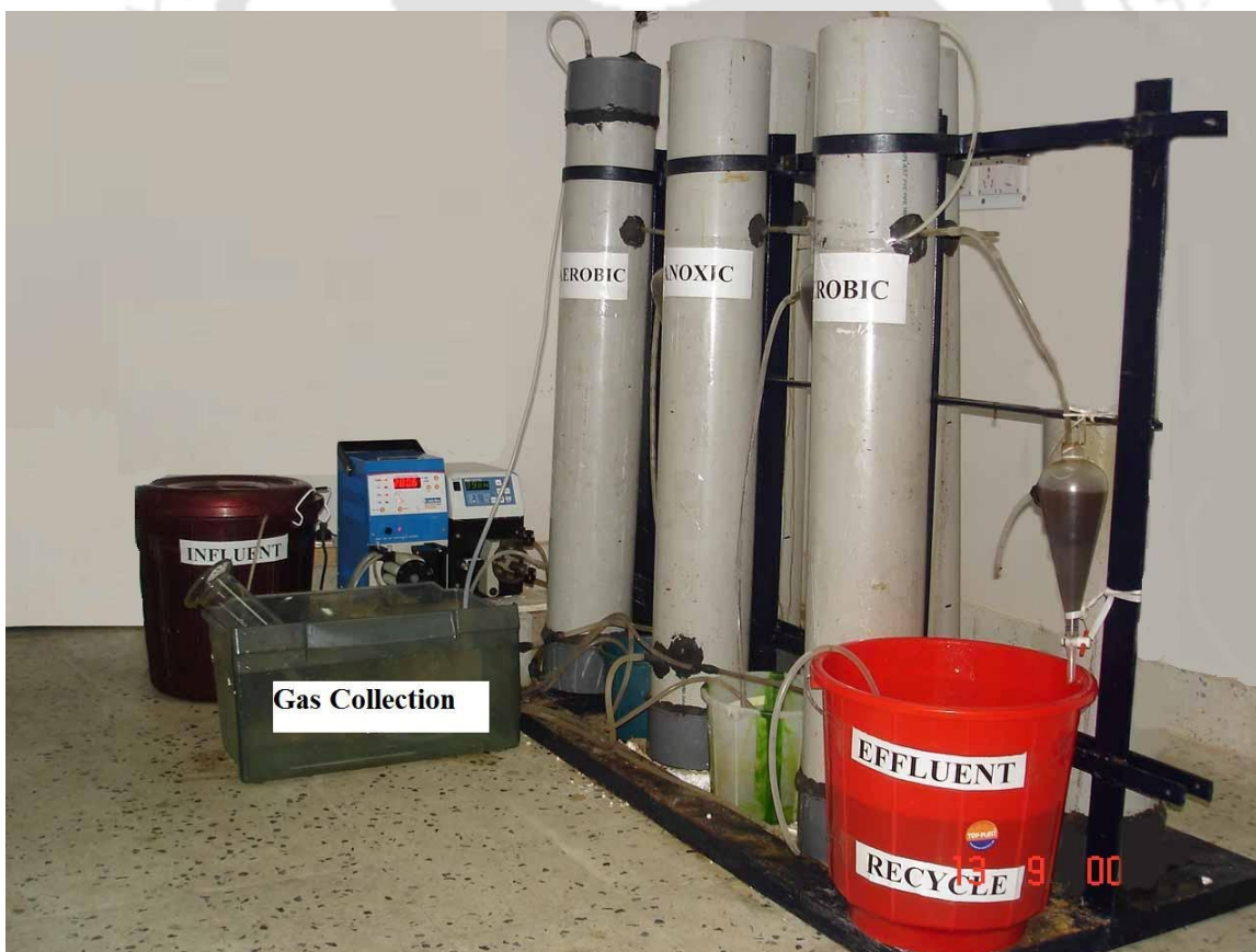
Figure 3.2 Photograph of the CMBR set up used in the study.
