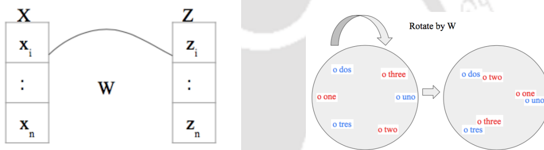
Figure 2.2: Learning a linear mapping matrix W from the entries of bilingual dictionary X (source language) and Z (target language), then rotate by W to align similar words across languages closer in a shared space
