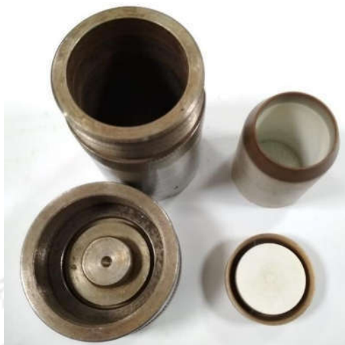
Figure 1.4 Image of the different parts of a Teflon-lined steel autoclave used in solvo/hydro-thermal reaction for the synthesis of MOF materials.
