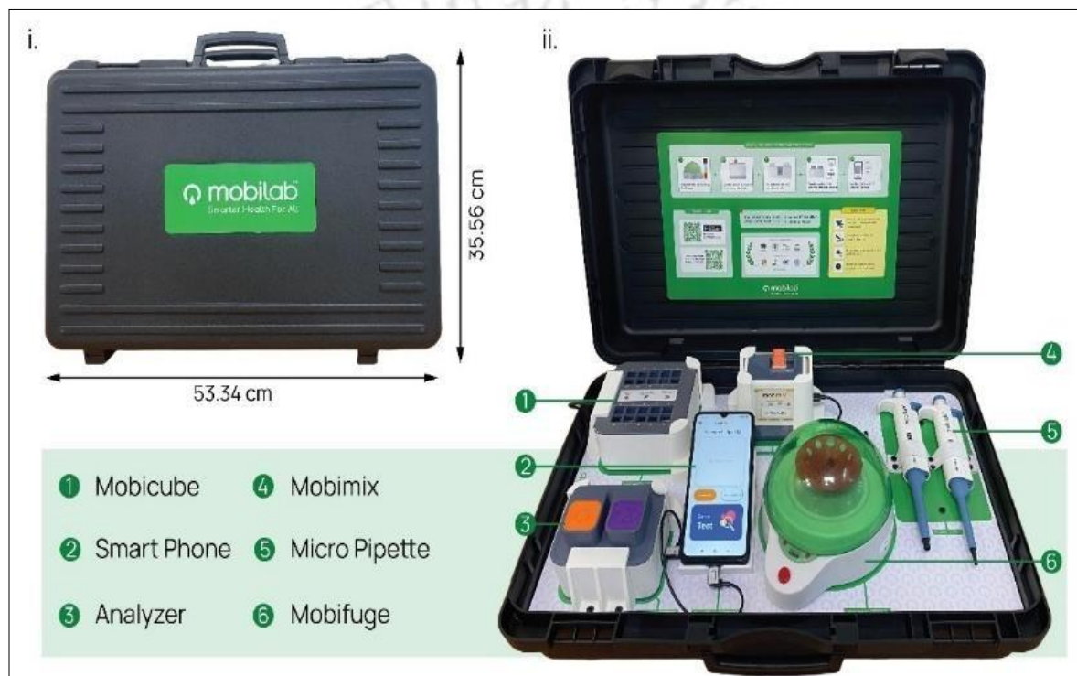
Figure 32. Mobicase: integrated portable kit for Mobilab-based point-of-care testing. (i) Closed view of the Mobicase, a portable carry unit measuring ~53.34 cm in length and 35.56 cm in height. (ii) Open view showing internal arrangement of components: (1) Mobicube – compact battery-powered incubator for simultaneous incubation of multiple samples; (2) Android smartphone running the “Mobilab Connect” app for device control and data processing; (3) Analyzer – battery-operated Mobilab unit connected via OTG cable for biochemical measurement; (4) Mobimix – automated mixer for uniform sample–reagent blending; (5) Micropipette – for precise sample and reagent dispensing; (6) Mobifuge – portable centrifuge for serum separation from whole blood.
