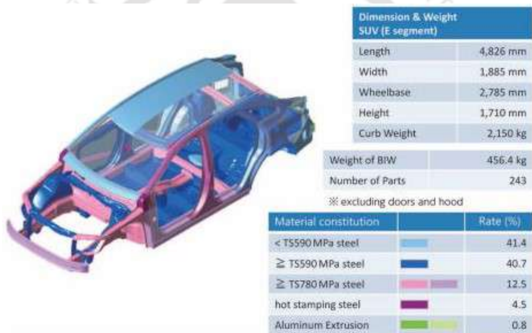
Fig. 1.1: Modern automobile body consisting multi-material (Naito and Suzuki [1])
