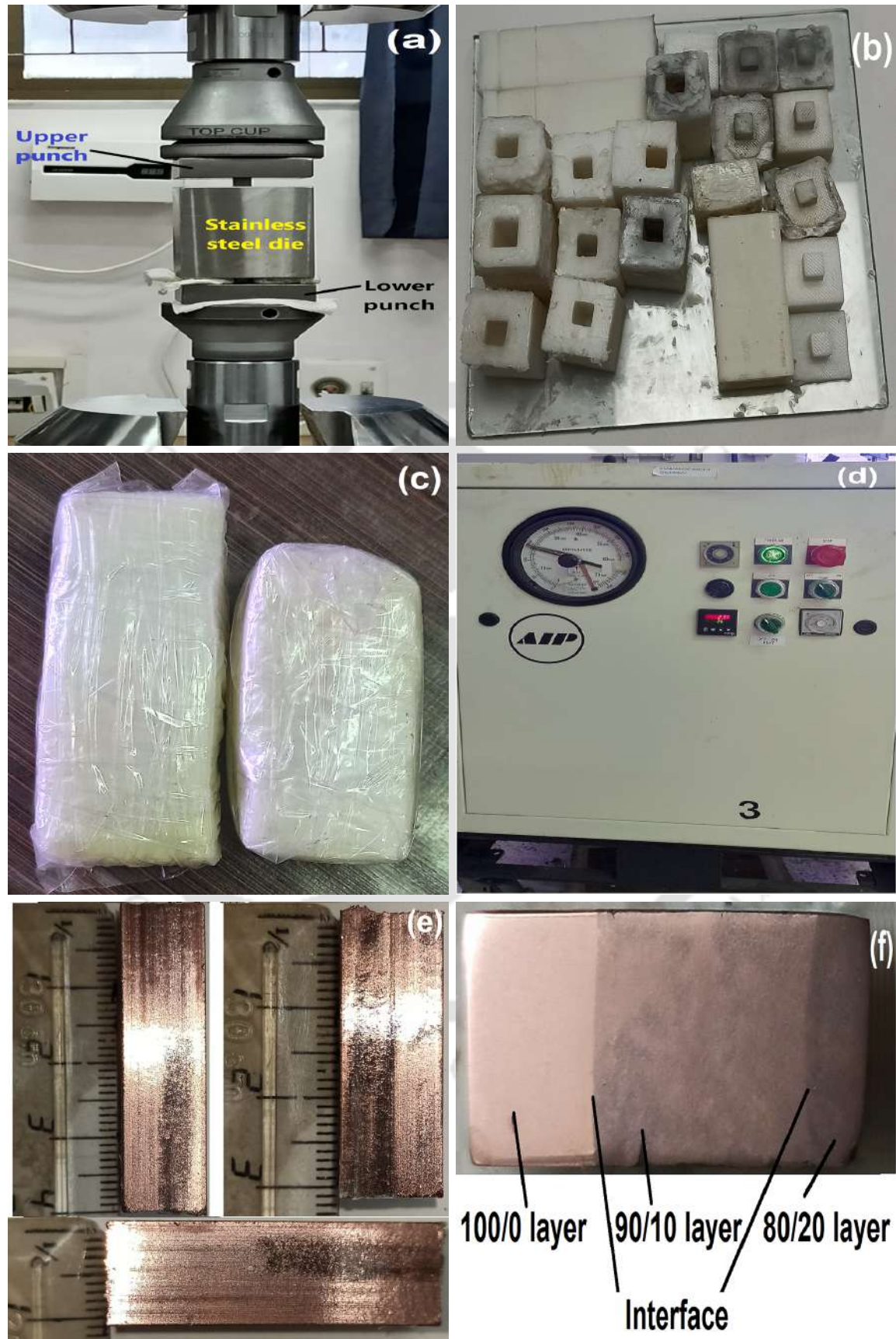
Fig. 6.2: (a) Uni-axial compaction at UTM (zoomed view) (b) Rubber molds (c) Sealed rubber mold for compaction (d) CIP unit (e) Cu/SiC green specimen (f) Sintered and polished specimen
