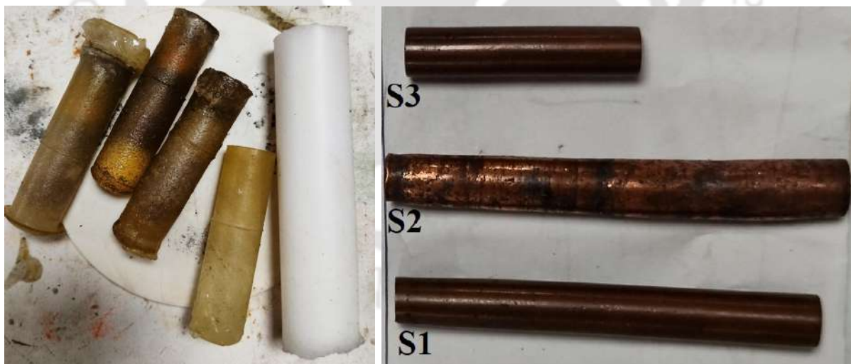
Fig. 7.1: (a) Cylindrical rubber mold and (b) Sintered Specimens
