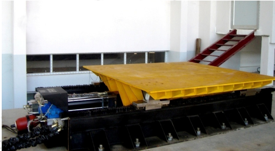
Fig. 3.2 Uni-axial Shaking Table (Make: BiSS, India)
