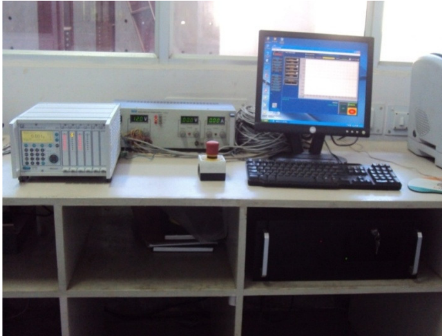
Fig. 4.5 Control system for the shake table testing
