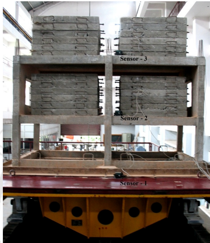
Fig. 5.3 Sensor locations in Model W-II during test
