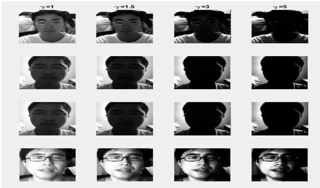
Figure 6.6: Impact of the Gamma power law on the degradation of the contrast profile of the original image (in the corresponding synthetic versions). Results are shown for \gamma = 1 ( no transformation) and for 1.5, 3, 5
