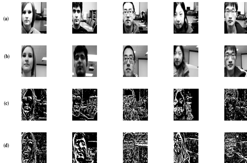
Figure 3.1: (a) Lowrank/Diffused component of attack face especially printed photo attack faces; (b) Lowrank/Diffused component of real legitimate faces; (c) Sparse/Specular component of printed photo attack faces; (d) Sparse/Specular component of real genuine faces. Images are taken from Wen et al. [2] printed photo database.
