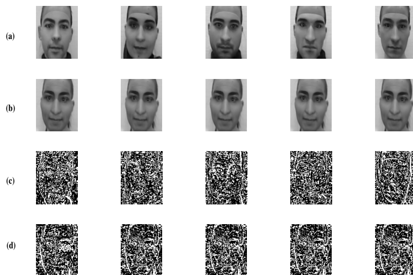
Figure 3.2: (a) Lowrank/Diffused component of spoofed faces wearing 3D masks; (b) Lowrank/Diffused component of real legitimate faces; (c) Sparse/Specular component of 3D mask faces; (d) Sparse/Specular component of real genuine faces.
