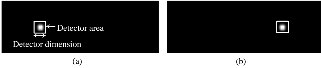
Figure 4.5: Synchronized movement of the detector area in the camera plane. (a) The first position of the beam on the camera surrounded by the detector area, and (b) another position of the beam on the camera again surrounded by the detector area.
