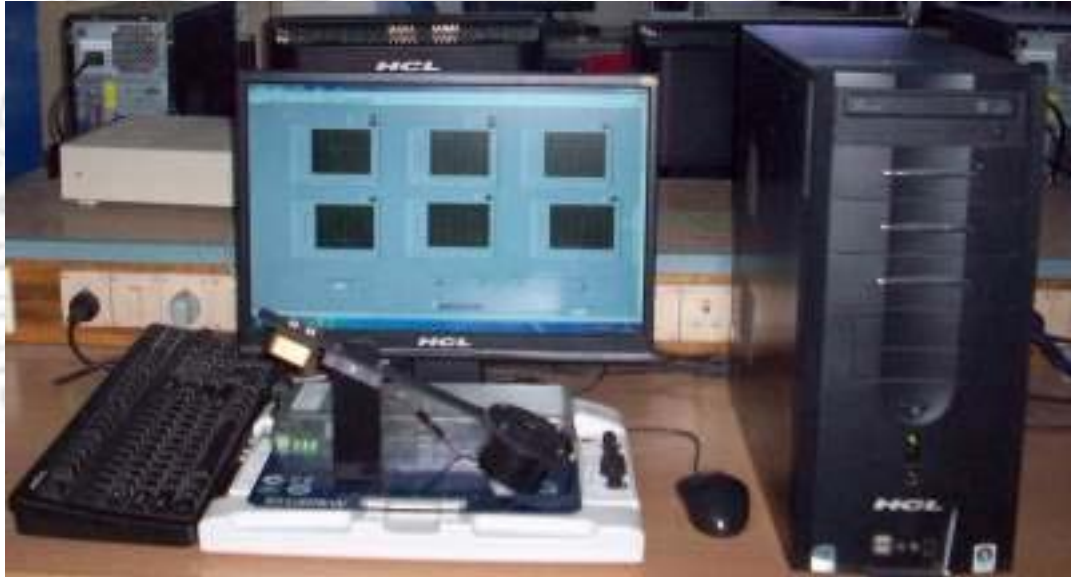
Figure 4.14: QNET VTOL trainer on ELVIS II
