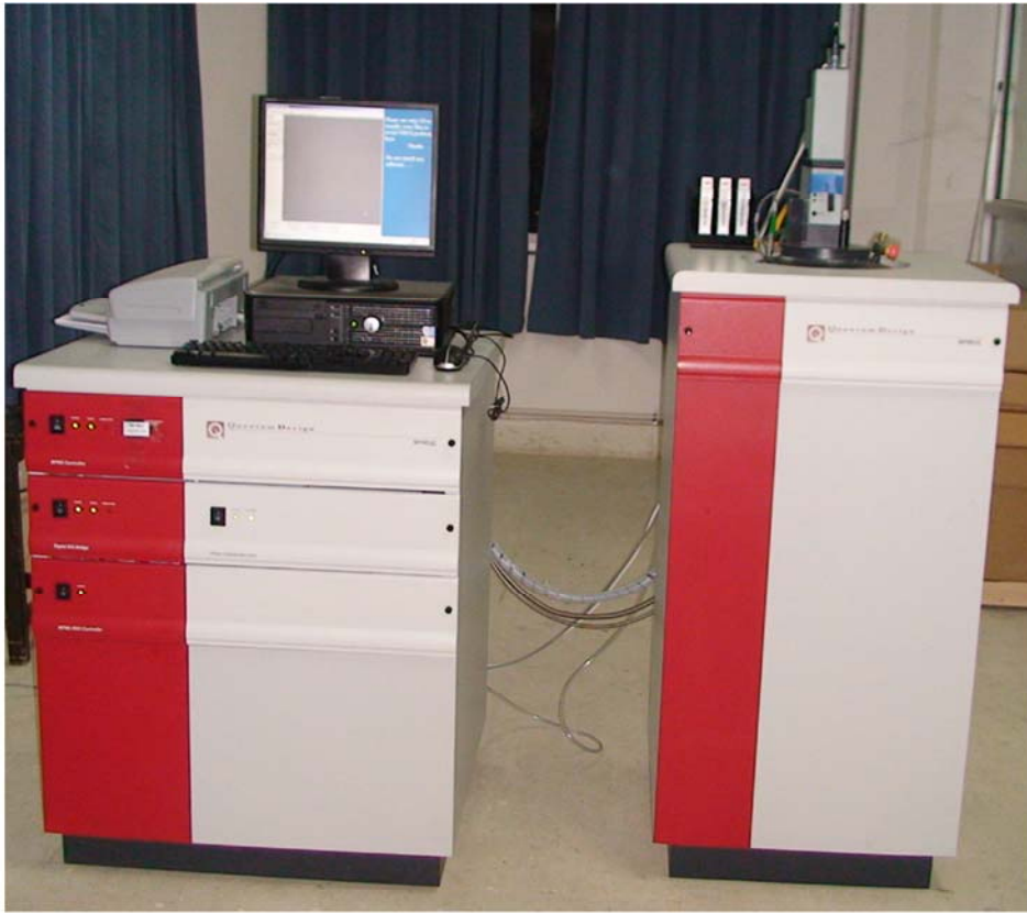
Figure 3.10: Photographic view of MPMS XL 7 system.
