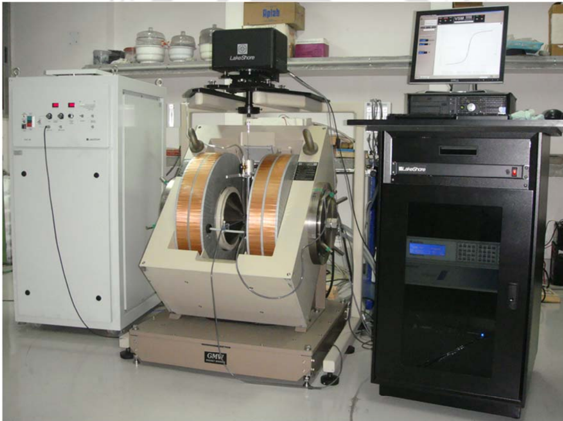
Figure 3.12: Photographic view of vibrating sample magnetometer (Model: Lakeshore 7410, USA) used in the present investigation.
