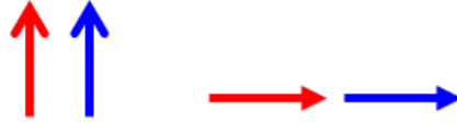
Figure 2.07: Schematic drawing of broadside and head-to-tail configurations for a pair of ferromagnetically coupled magnetic moments.
