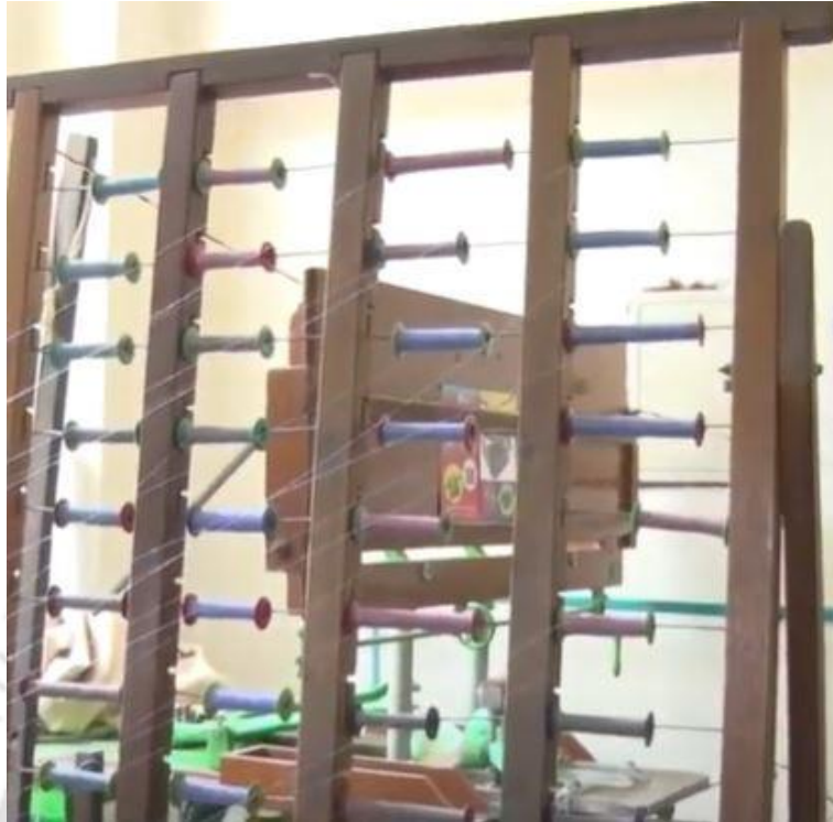
Figure 2.17: Wooden creel used in warping[33]
