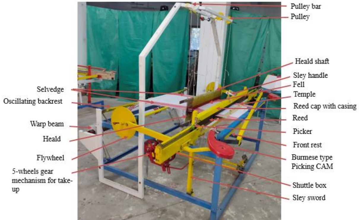
Figure 4.95: De-sign semi-automatic handloom without jacquard (beta model) from the left front at DoD, IIT Guwahati workshop
