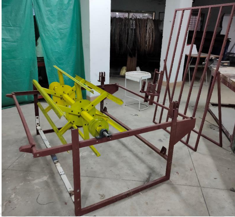
Figure 5.15: Warping drum with creel (Pre-weaving tools) with sheet metal formed mild steel structure
