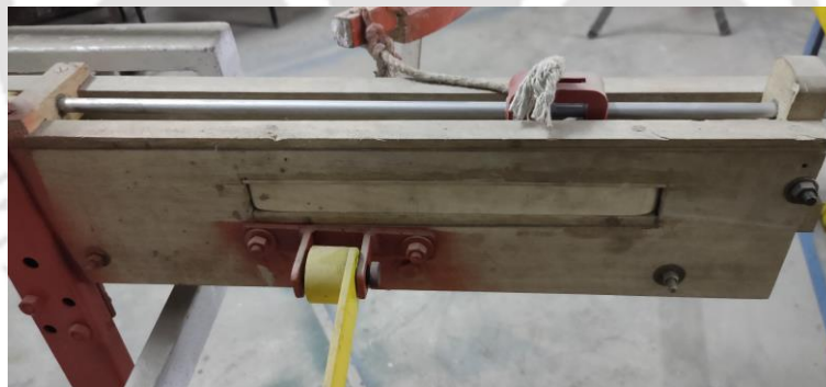
Figure 4.22: Left side Shuttle box with spring action
