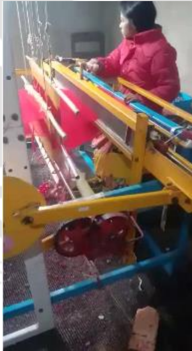
Figure 6.47: Semi-automatic handloom on production on another site
