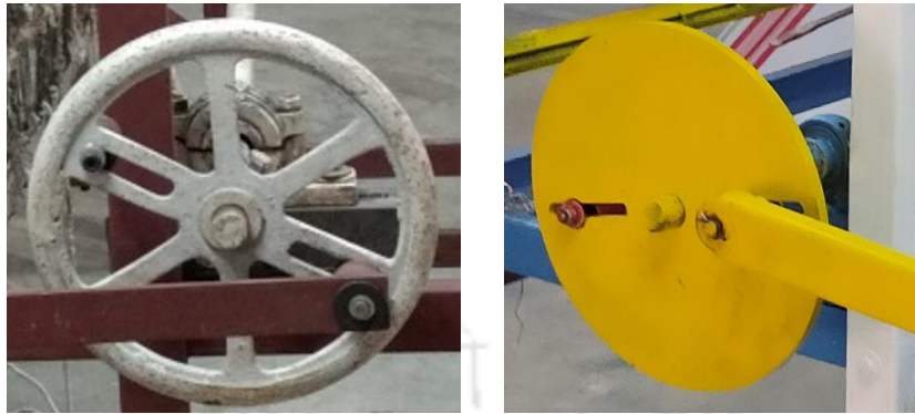
Figure 6.13: Comparison of the flywheel in alpha and beta model
