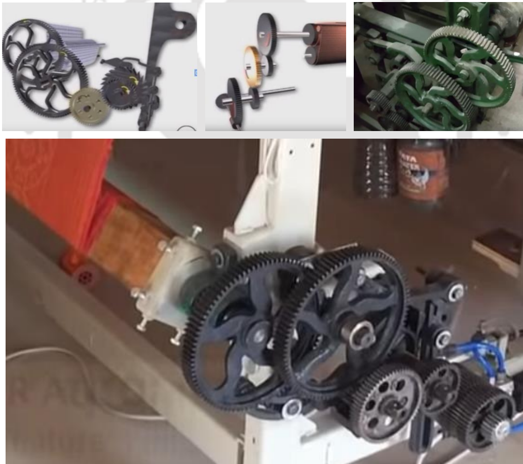
Figure 4.53: Existing Gear mechanisms for take-up motion
