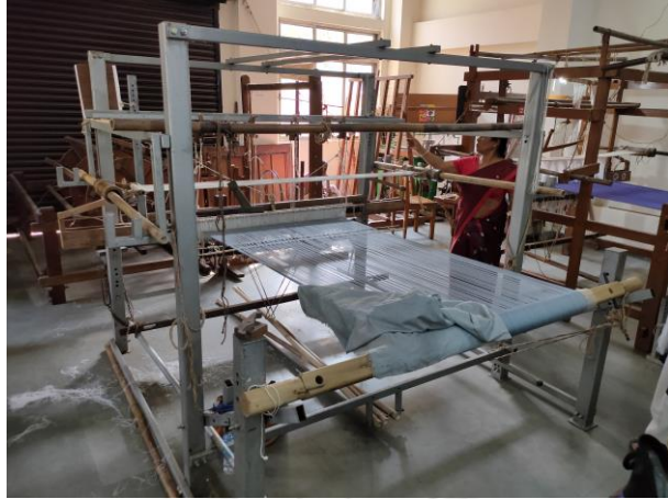
Figure 2.33: Metal frame fly-shuttle handloom at Handloom development research centre, Ambari, Guwahati
