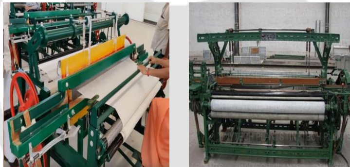
Figure 2.47: Automatic solar and manual pedal convertible loom
