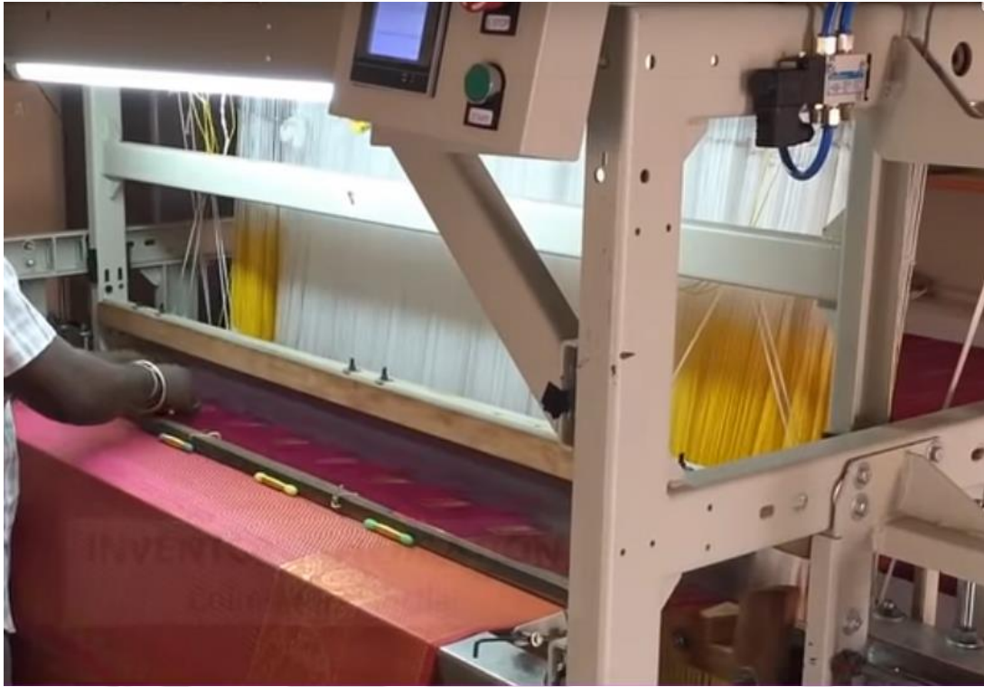
Figure 2.49: Automatic sheet metal pneumatic handloom
