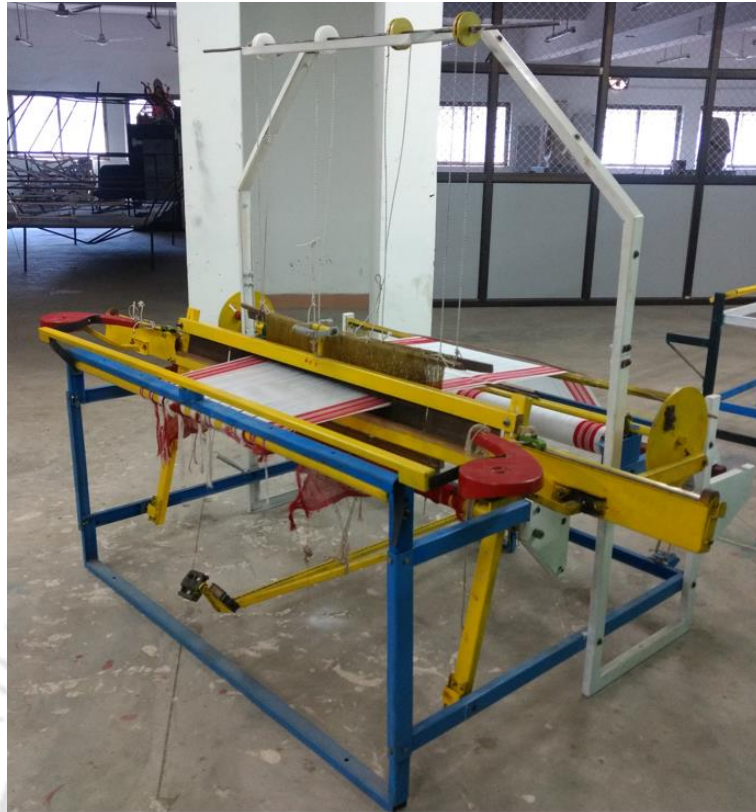
Figure 4.96: Design semi-automatic handloom without jacquard (beta model) from the right front at DoD, IIT Guwahati workshop
