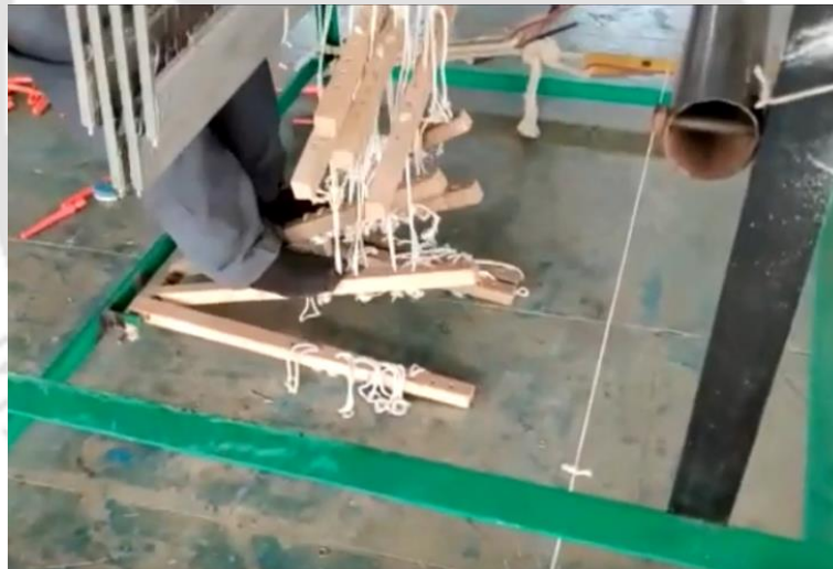
Figure 2.37: Jack and Lam loom with front side pivot
