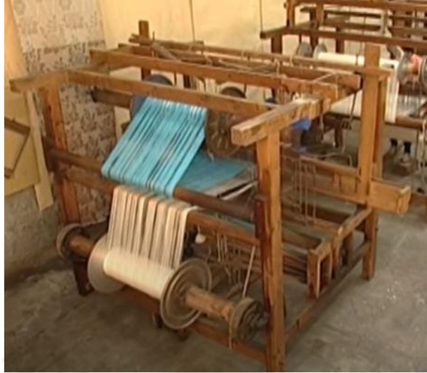
Figure 2.38: Extra warp handloom with terry towel weaving capability
