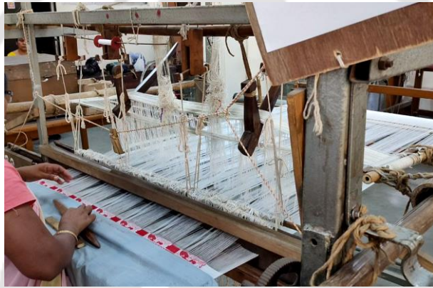
Figure 2.34: Metal frame fly-shuttle handloom with dobby at Handloom development research centre, Ambari, Guwahati
