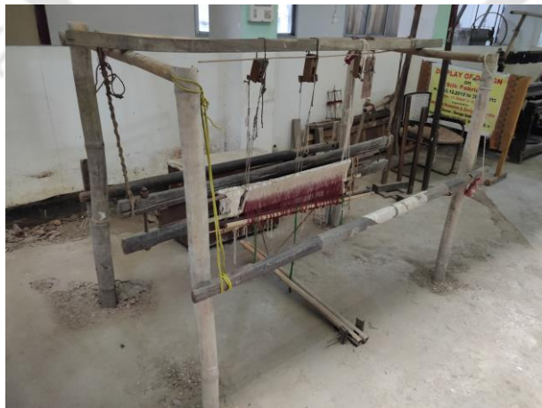
Figure 2.35: Bamboo frame through-shuttle handloom at Handloom development research centre, Ambari, Guwahati
