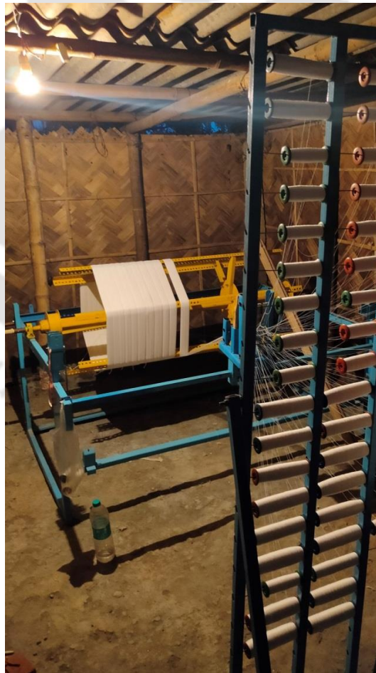
Figure 5.16: warping drum with creel at customer location
