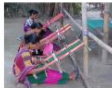
Traditional loom is low productive, tedious primitive handloom uses loin of the weaver and upper limbs for weaving.
