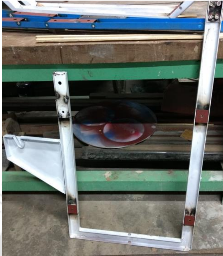
Figure 6.14: Side frame with 2mm sheet thickness and 50mm width
