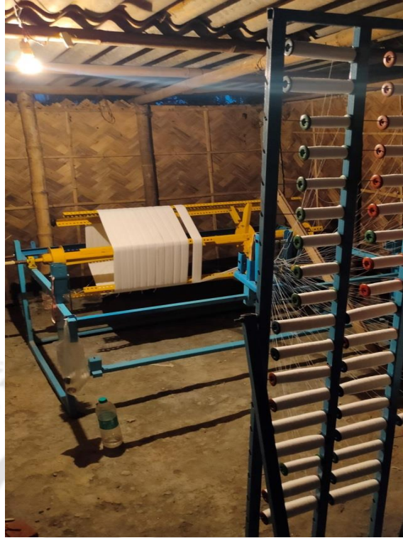
Figure 6.46: warping drum with creel at customer location
