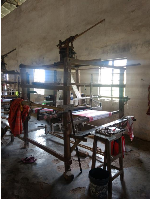
Figure 2.31: Wooden frame fly-shuttle handloom with jacquard at ARTFED, Guwahati
