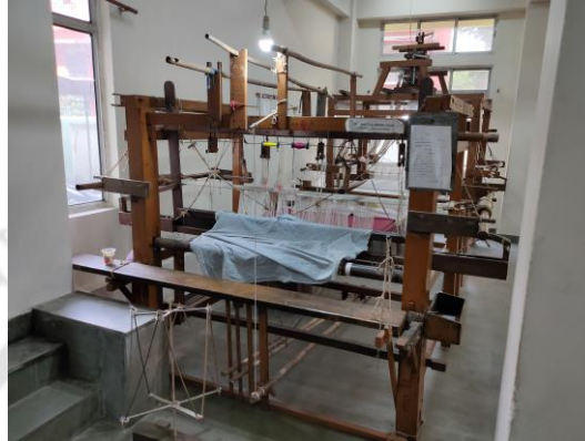
Figure 2.29: Wooden frame fly-shuttle handloom without jacquard at Handloom development research centre, Ambari, Guwahati
