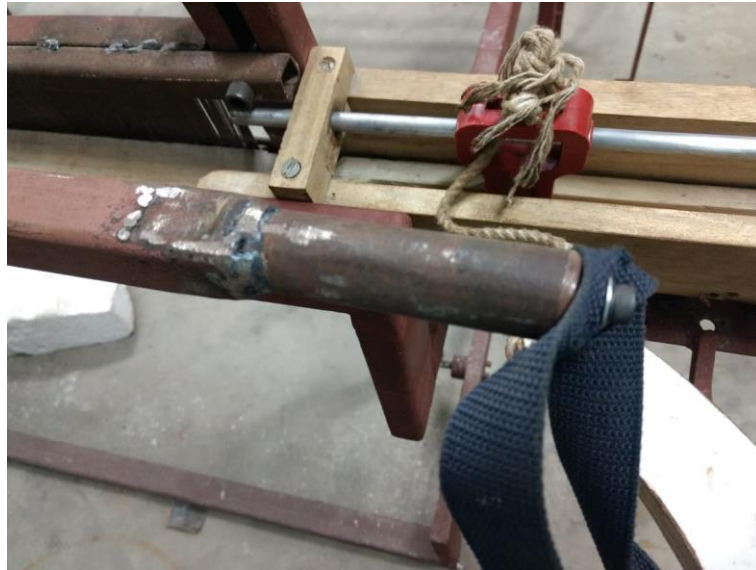
Figure 4.52: CAM to picker connection in the alpha model of semi-automatic handloom
