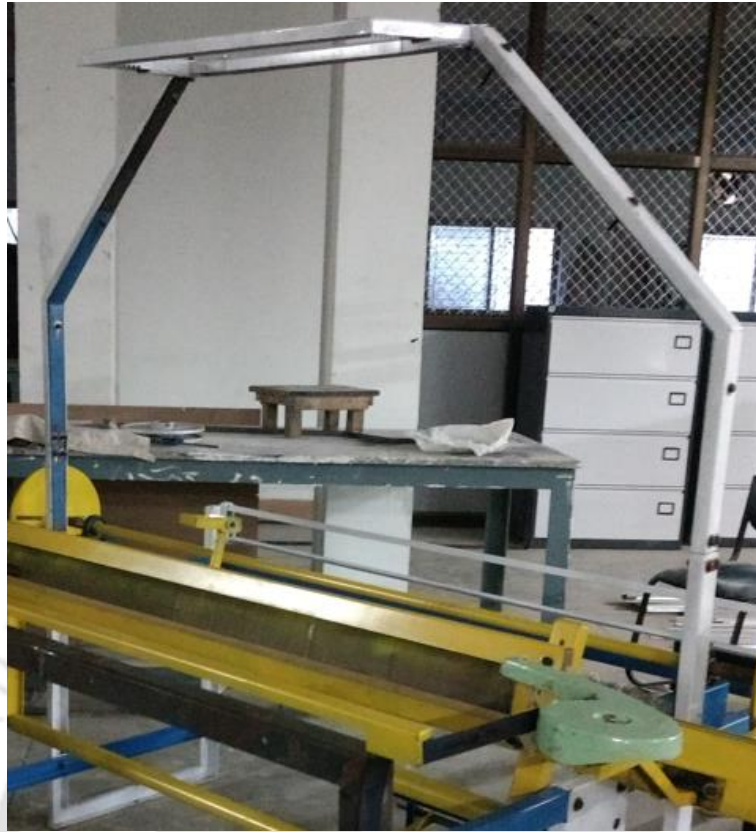
Figure 6.16: Side frame with full reinforcement
