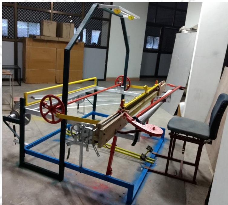
Figure 4.51: Manufactured alpha model of semi-automatic handloom 2
