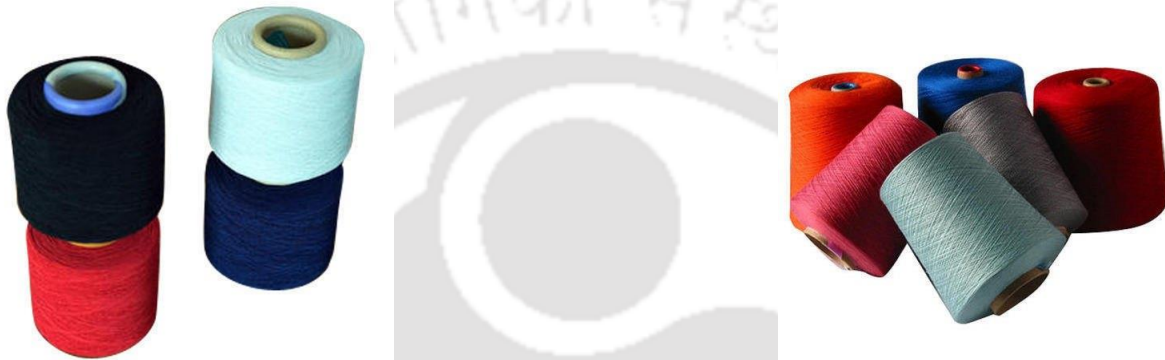
Figure 2.10: Yarn in Cop form Figure 2.11: Yarn in Cone form (for handloom weaving)
