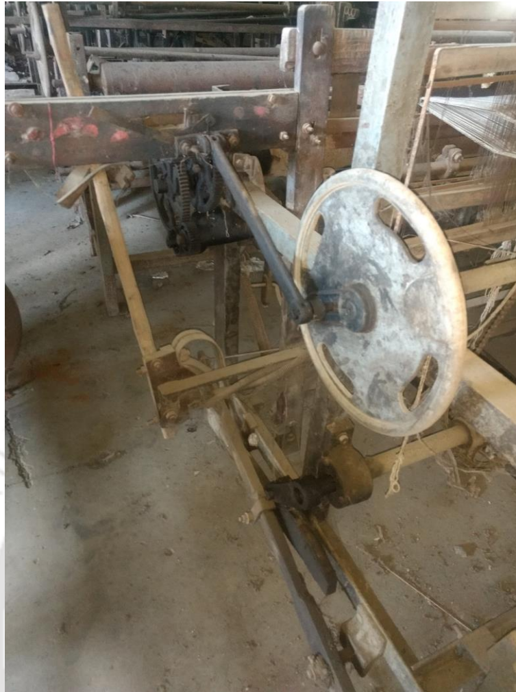
Figure 4.1: Metallic mechanism in wooden sley in fly-shuttle handloom
