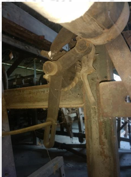
Figure 2.52: Actuator in take-up gear mechanism in semi-automatic handloom at ARTFED, Guwahati
