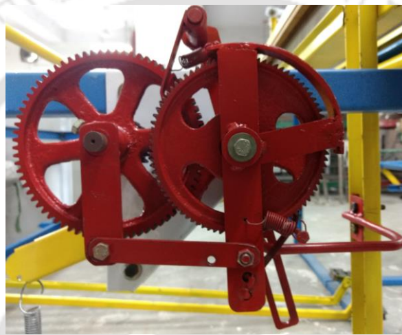
Figure 6.11: Front view of 5-wheel gear mechanism in beta model
