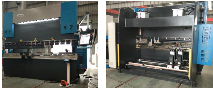
Figure 4.87: Front and Rear view of CNC bending machine
