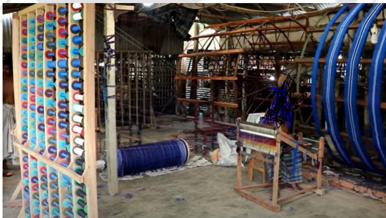
Figure 2.21: Set of Creel and Warping drum with warp beam[34]
