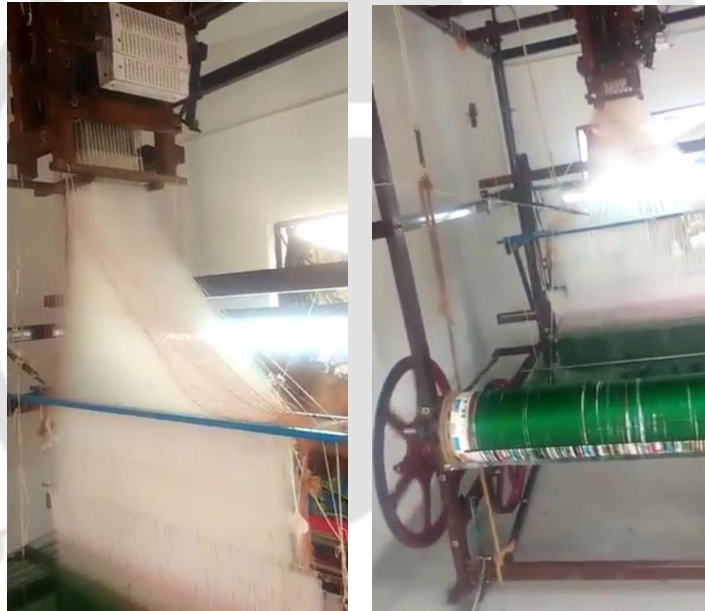
Figure 2.44: Semi-automatic handloom with automated shedding, manual picking, and beat up at Tamilnadu [15]
