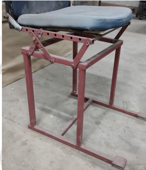
Figure 5.17: Alpha-model of a seating system for handloom
