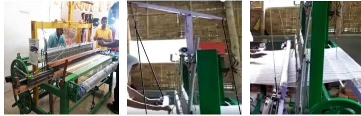
Figure 2.48: Paddle-operated semi-automatic handloom
