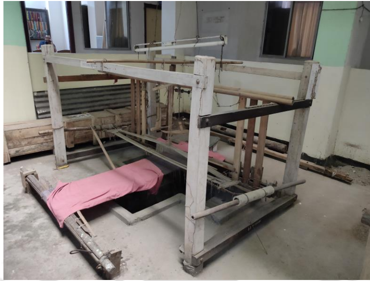
Figure 2.36: Wooden throw-shuttle pit handloom at Handloom development research centre, Ambari, Guwahati
