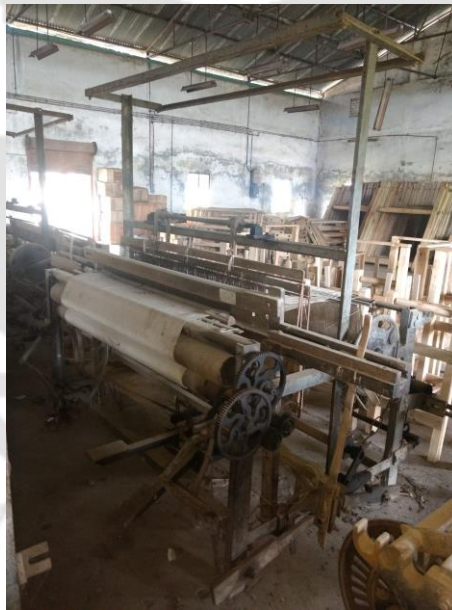
Figure 2.46: Semi-automatic handloom at ARTFED, Guwahati
