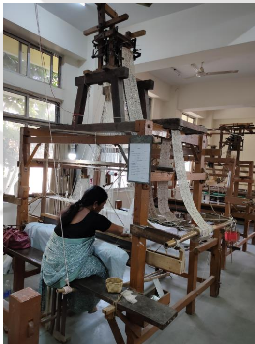
Figure 2.30: Wooden frame fly-shuttle handloom with jacquard at Handloom development research centre, Ambari, Guwahati
