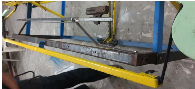
Figure 4.33: Temple mounting with right side spring roller temple in Semi-automatic handloom
