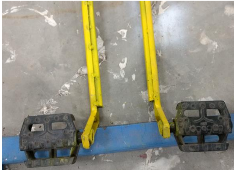
Figure 6.2: Sheet metal treadle with reinforcement
