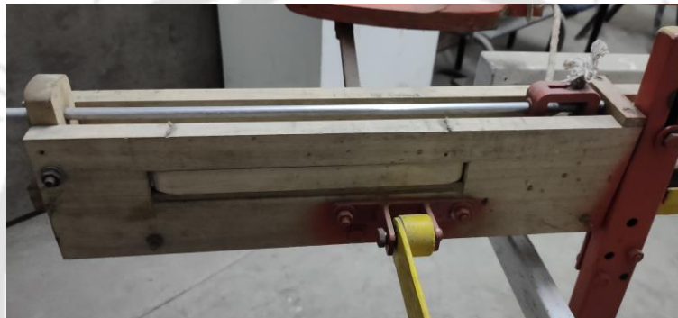
Figure 4.21: Right side Shuttle box with spring action
