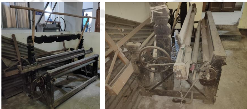
Figure 2.41: Chittaranjan semi-automatic handloom at Handloom development & research centre, Ambari, Guwahati
