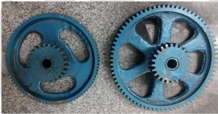
Figure 4.55: Compound gear of 5-wheel gear in the alpha model of semi-automatic handloom
