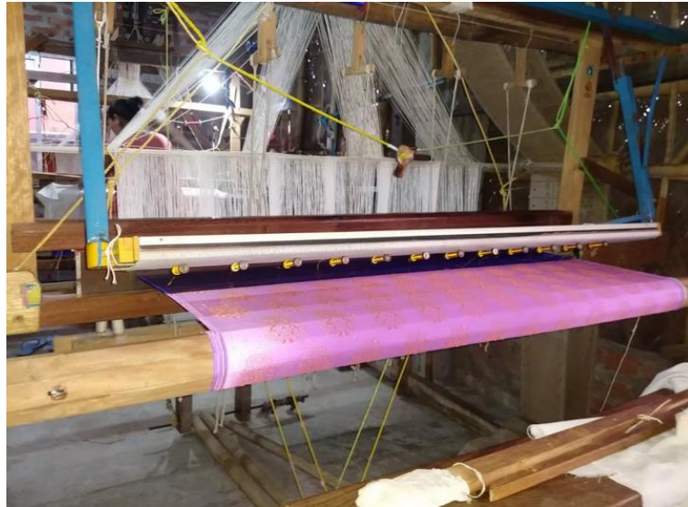
Figure 2.40: Buta machine with sley in handloom
