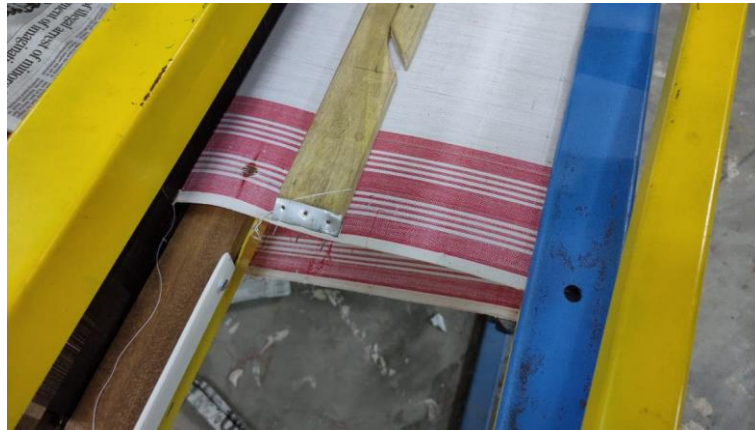
Figure 4.57: Wooden temple motion in the alpha model of semi-automatic handloom
