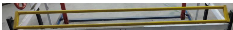
Figure 4.35: Oscillating backrest with the round tube of the alpha model of semi-automatic handloom
