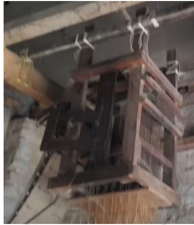
Figure 2.53 Wooden Jacquard model with less metal
