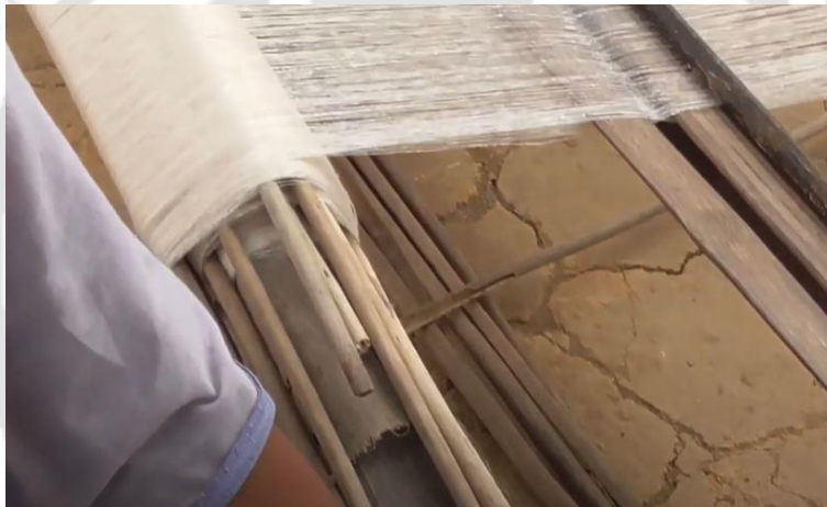
Figure 2.14: Pre weaving activity - 1 on Warp beam[15]
