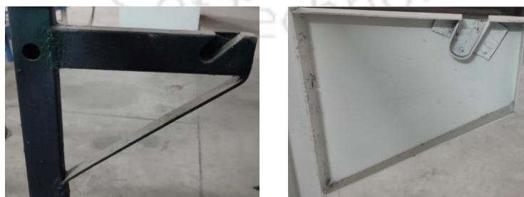
Figure 4.78: Warp beam holding bracket comparison in alpha and beta model
