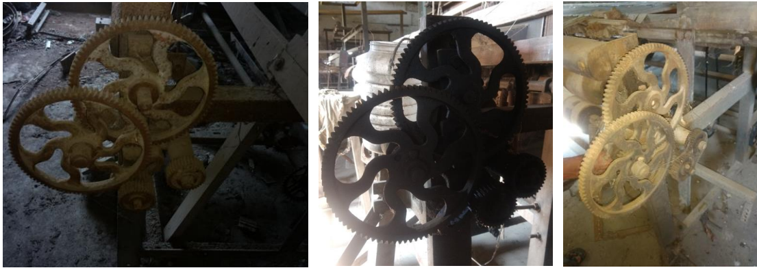
Figure 2.51: Gear mechanism in semi-automatic handloom at ARTFED, Guwahati
