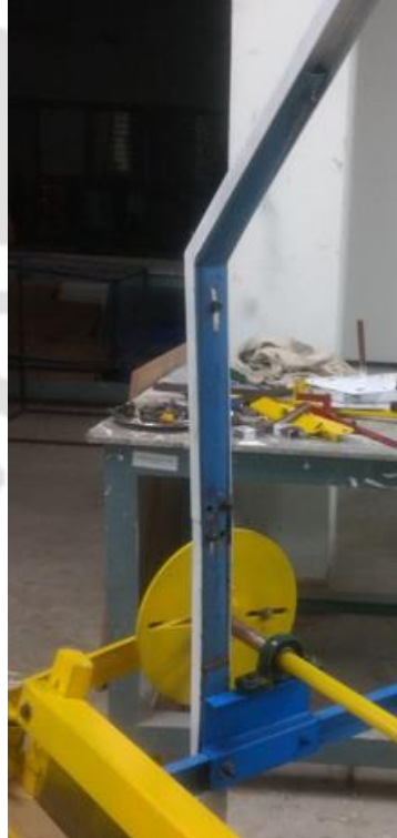
Figure 6.15: Side frame with 2mm sheet thickness along with reinforcement
