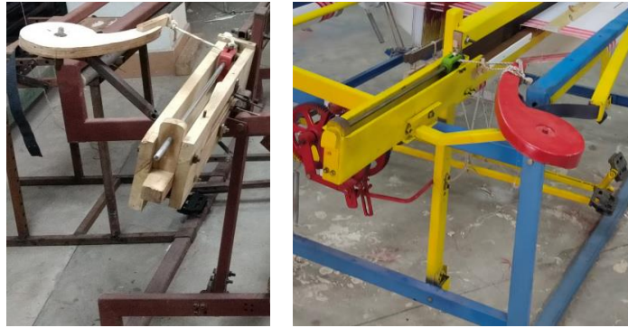
Figure 6.6: Comparison of Cam mechanism for picking in alpha and beta model
