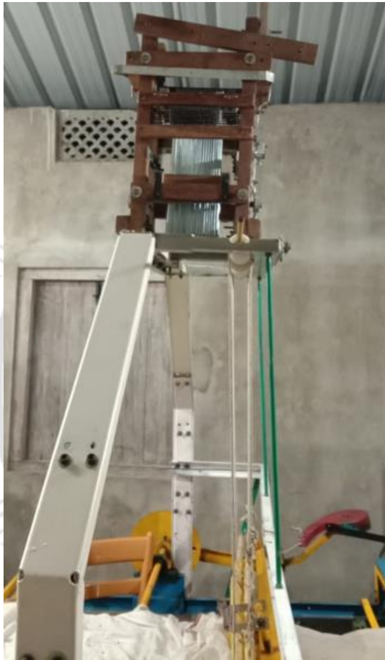
Figure 5.19: Semi-automatic handloom with wooden frame jacquard
