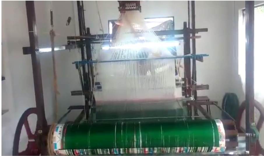
Figure 2.43: Semi-automatic handloom (shedding) is automated, manual picking and beat up) at Tamilnadu [15]
