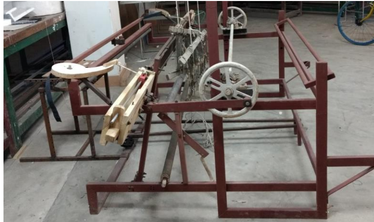
Figure 4.50 Manufactured alpha model of semi-automatic handloom
