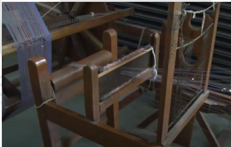
Figure2.18: Wooden hack frame between creel and warping drum used in warping[33]
