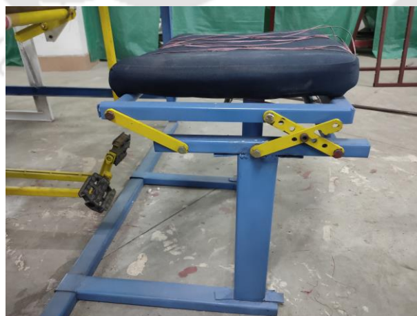
Figure 5.18: Seating system for semi-automatic handloom
