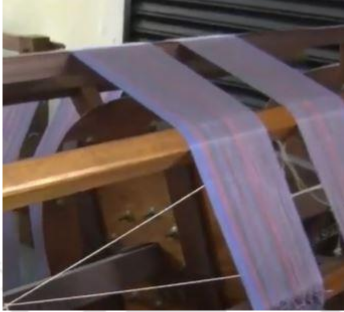
Figure 2.19: Wooden warping drum used in warping - 1[33]
