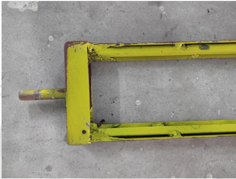
Figure 6.20: Sheet metal structured with an additional square bar in the oscillating backrest
