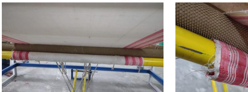
Figure 6.12: Slippage of thin fabric in cloth beam
