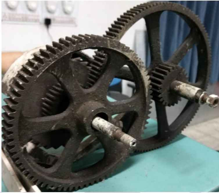
Figure 4.54: Re-organisation concept of the 5-wheel gear train with two shafts for take-up and let-off motions
