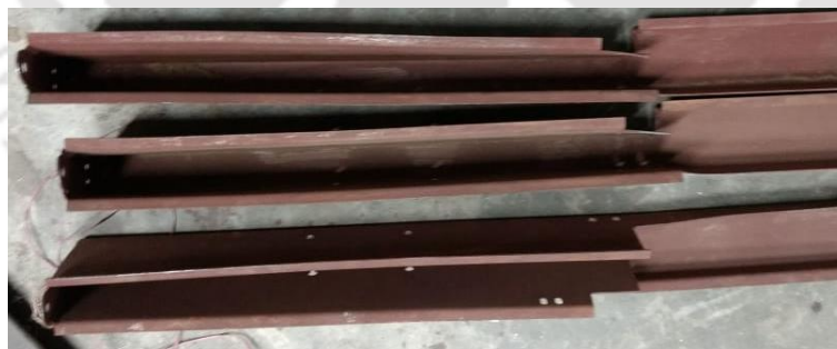
Figure 6.25: Damaged sheet metal component during transportation
