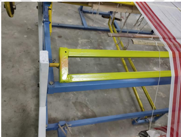
Figure 6.22: 1" square tube structured in the oscillating backrest
