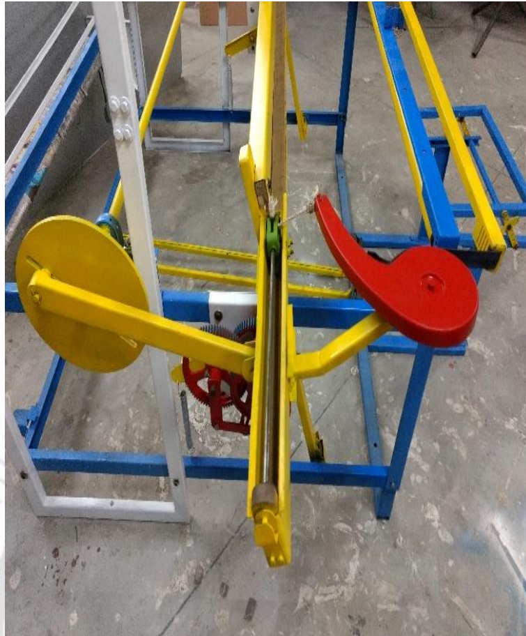
Figure 4.98: Enlarged view of Picking and beat-up mechanism
