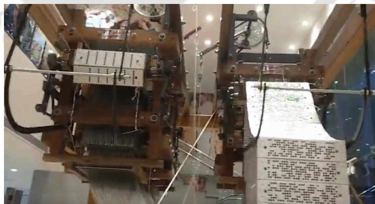
Figure 2.39: Double jacquard mounted on a single loom
