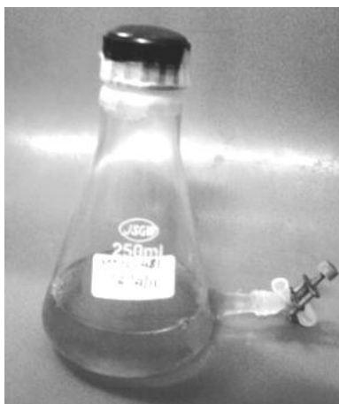
Figure 4.3: Custom fabricated flask with a bottom spout and screw cap for anaerobic clostridial cultures
