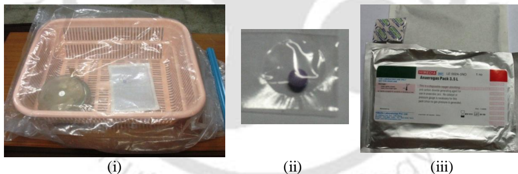
Figure 4.2: Anaerobic culturing of clostridial species. (i) Anaero bag, (ii) Anaero indicator tablet, (iii) Anaerogas Pack
