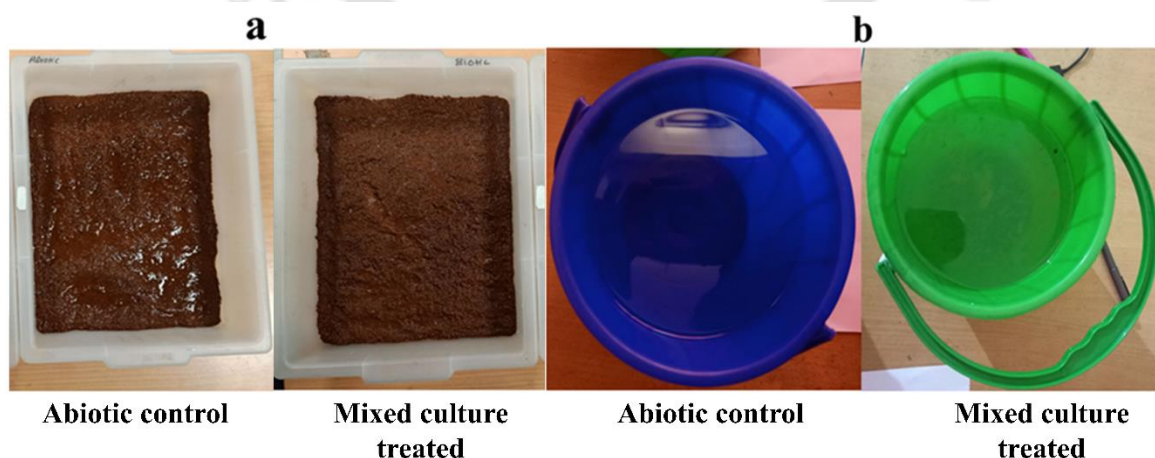
Fig. 7.1. Experimental setup for diesel degradation studies in soil and water: (a) Trays for soil degradation: the left tray represents the abiotic control (no bacterial
