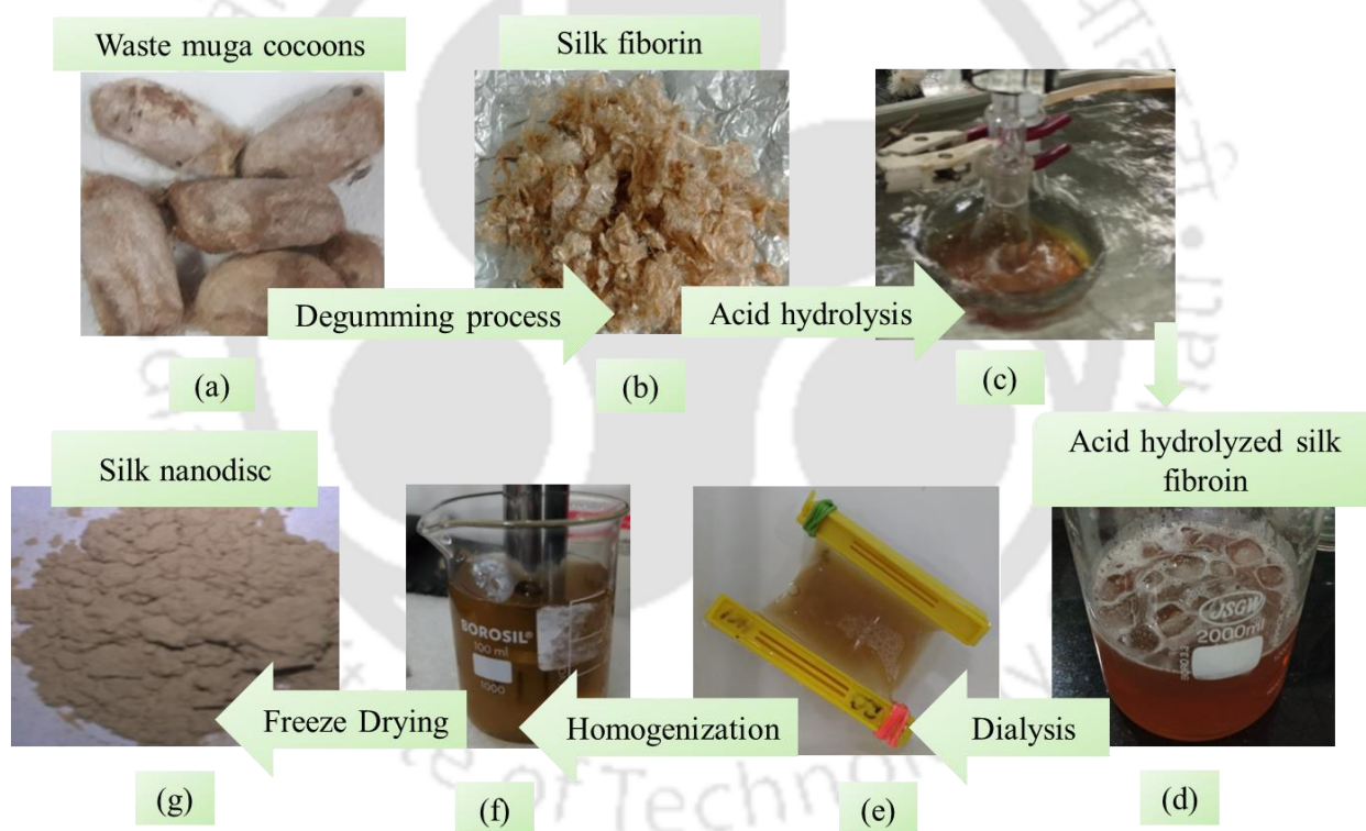
Figure 2.3 Fabrication of silk nanodisc using acid hydrolysis method representing (a) Waste muga cocoons; (b) Silk fibroin (degummed silk); (c) Acid hydrolysis of silk fibroin; (d) Acid hydrolysed silk nanodisc; (e) Dialysis of acid hydrolysed silk nanodisc; (f) Homogenization of silk nanodisc; and (g) Freeze dried silk nanodisc.
